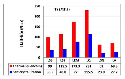
Figure 9. Half-life values of tensile strength of limestones under cyclic thermal and salt weathering.
