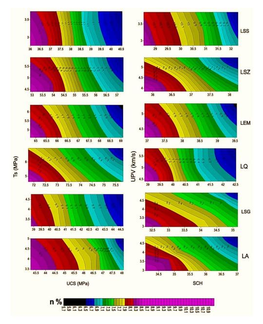
Figure 4. Influence of porosity (n) on TS, UCS, UPV, and SCH for the tested limestone specimens.
