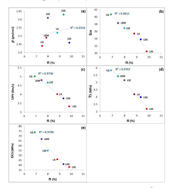
**Figure 3.** Relationship between porosity, n (%) and (**a**) desity,  $\rho$  (gm/cm<sup>3</sup>), (**b**) Shmidt hammer rebound, SCH, (**c**) ultra sound pulse velocity, UPV (Km/s), (**d**) tensile strength, Ts (MPa), and (**e**) uniaxial compression strength, UCS (MPa).
