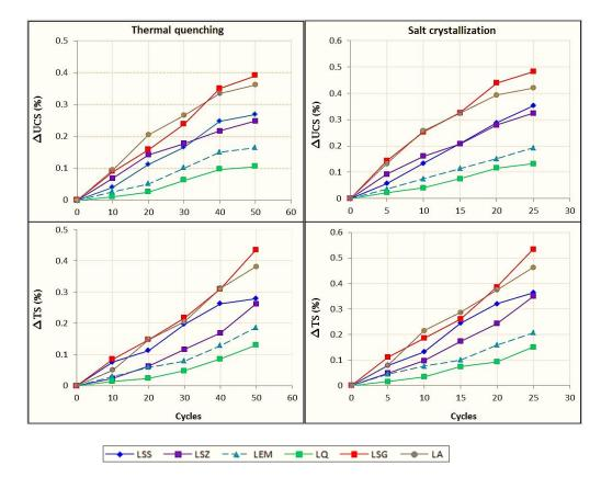
Figure 7. Change rate of TS and UCS values due to the cyclic thermal quenching and salt crystallization.
