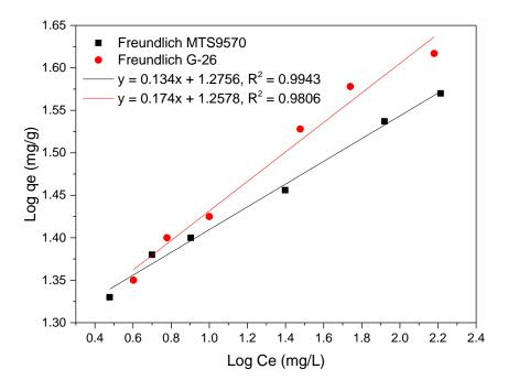
Figure 9. Freundlich isotherm of Pb(II) adsorption on G-26 and MTS9570.
