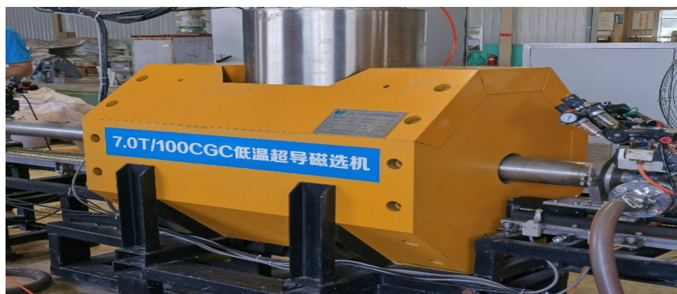
Figure 1. The 7.0T/100CGC low-temperature superconducting magnetic separator used in this study.
