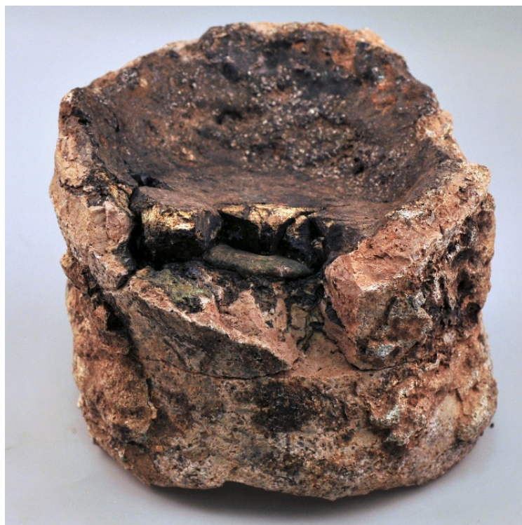
Figure 3. Crucible from Svor with dark blue glass layer.
