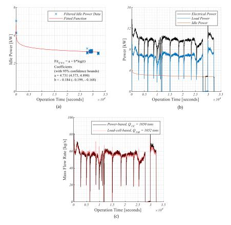
**Figure 4.** (a) Model fitting in idle power data set for conveyor  $CV_1$ , (b) Calculated load power signal for conveyor  $CV_1$ , (c) Calibrated power-based mass flow rate signal for conveyor  $CV_1$ .
