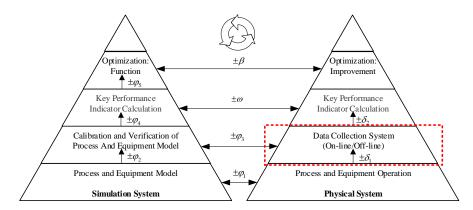
Figure 1. Error propagation model for the implementation of the optimization functionality in crushing plants [1,9].
