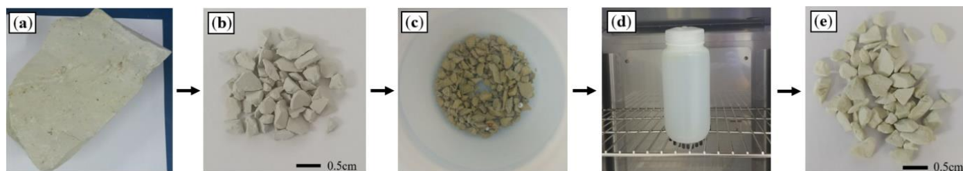
Figure S2. The “top-down” synthesis approach to produce granular-sized zeolites: (a) natural zeolite ore, (b) crushed natural zeolite (granular-sized), (c) zeolite immersed in NaOH solution, and (d) during the reaction process in the oven, and (e) resulting as-synthesized NaP zeolite (granular-sized).
