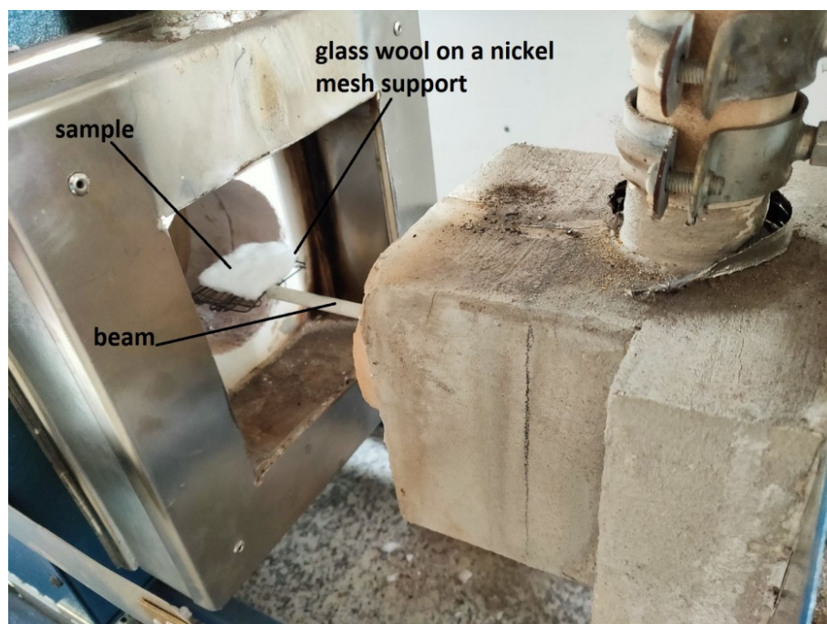
Figure 2. Method of placing a test sample on an electronic weighing pan [12].
