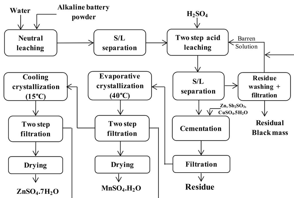
**Figure 2.** Chemical leaching flow sheet of Zn and Mn extraction from alkaline battery (redrawn and adapted with modifications from [62]).
