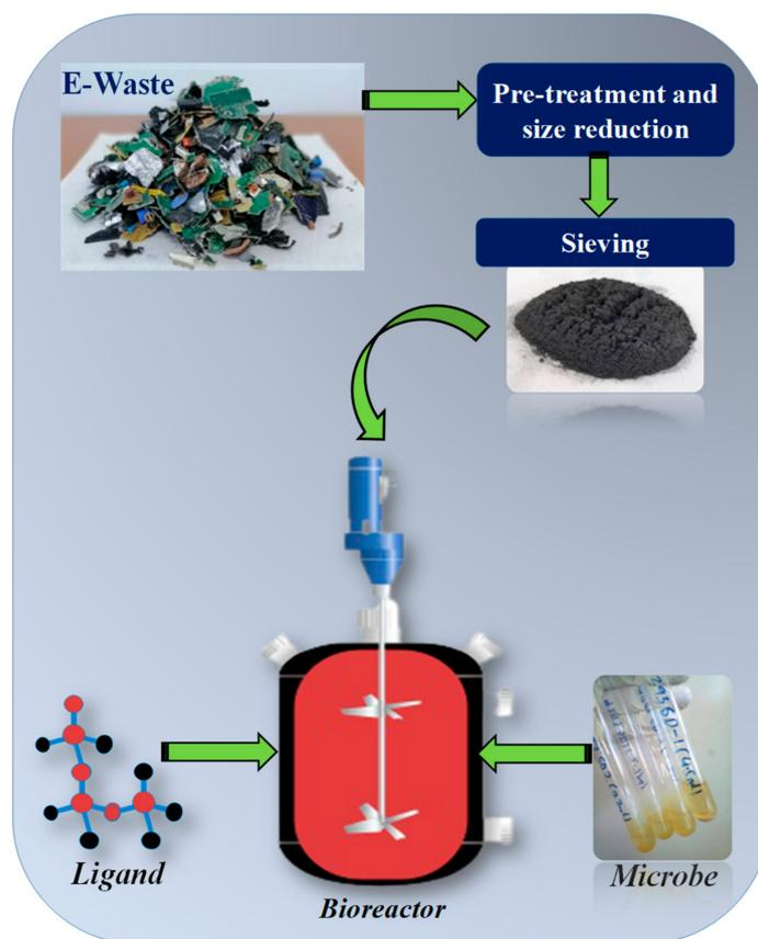
**Figure 7.** Pictorial representation of a ligand mediated integrated bioleaching approach.
