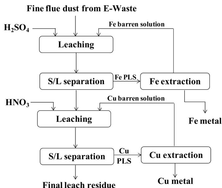
Figure 4. Metal leaching from e-waste flue dust (redrawn with modifications following [30]).
