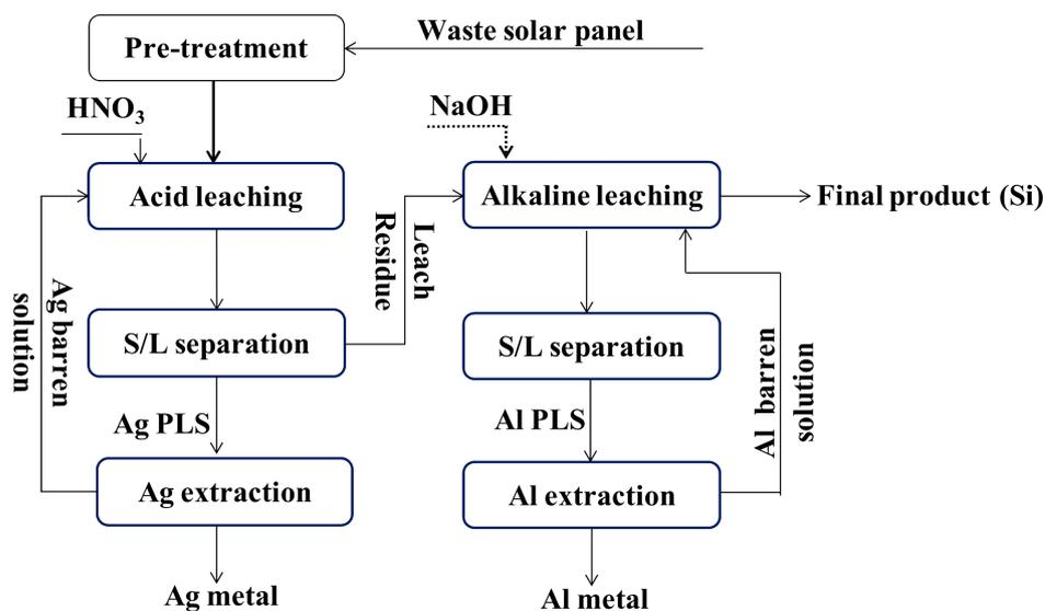
**Figure 3.** A typical flow sheet for metal leaching from solar panels (Drawn following information from [65,79]).
