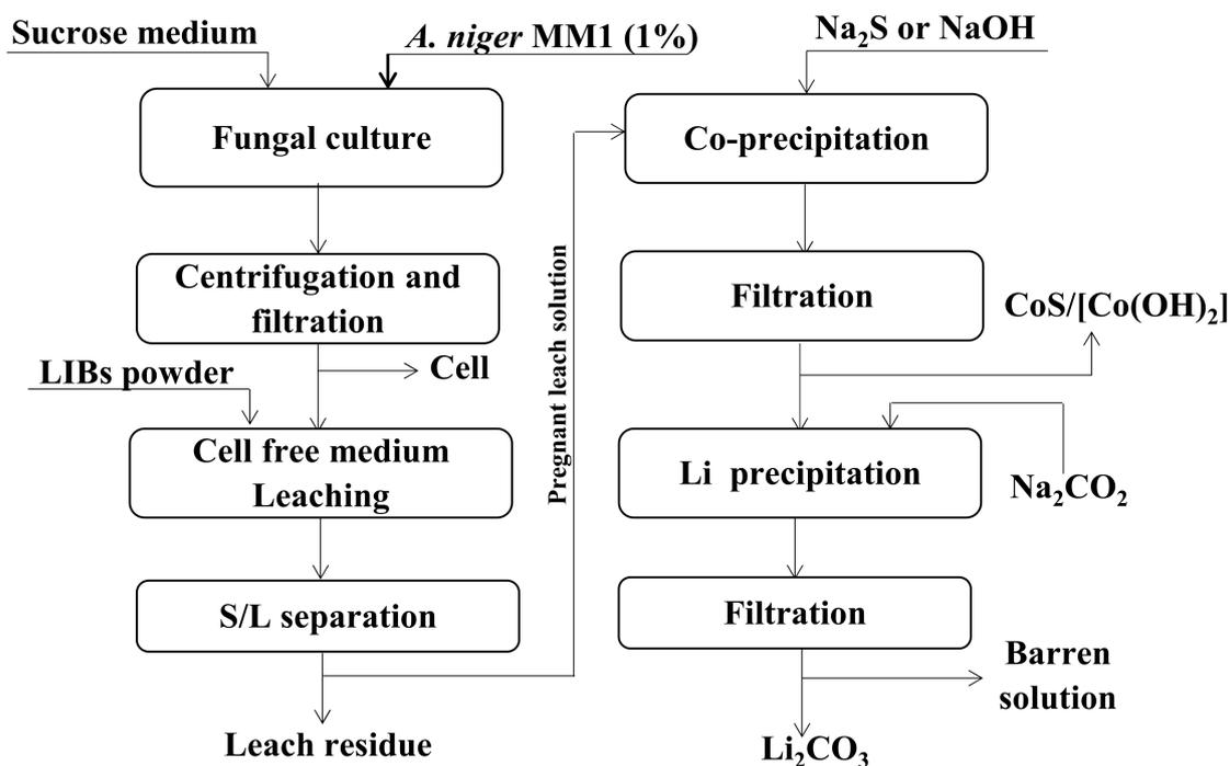
Figure 6. Bioleaching of LIBs with *A. niger* (drawn based on information collected from [112]).
