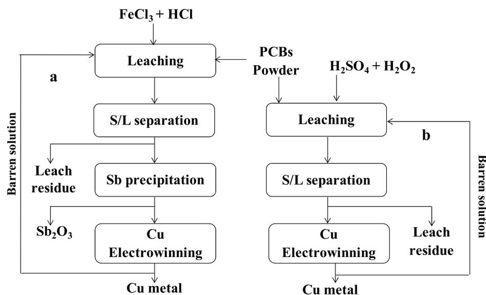
**Figure 1.** Cu metal recovery from waste PCBs. The flow sheet is drawn following information collected from (a) [31], (b) redrawn following [33].
