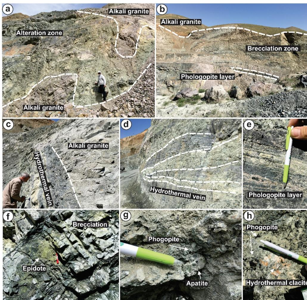
**Figure 3.** Photographs of field observation in the Ghareh Bagh mica mine. (a,b) A Ghareh Bagh mica mine pit. Photos show Ghareh Bagh mine located in alkali granite in the breccia zone with the high alteration. Mine is as layer trended in NW-SE. (c,d) Hydrothermal vein including the matrix of chlorite, biotite, actinolite, K-feldspar, calcite and quartz. (e) Phlogopite layer with NW-SE. (f–h) Coarse-grained minerals in parageneses of phlogopite in breccia are epidote, apatite and calcite.
