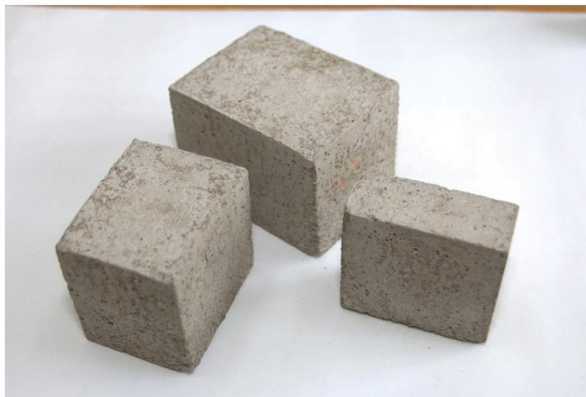
**Figure 11.** Concretes from magnesium-containing rocks of the Yoko–Dovyren massif. Large one have size  $20 \times 12 \times 10 \text{ cm}^3$ .
