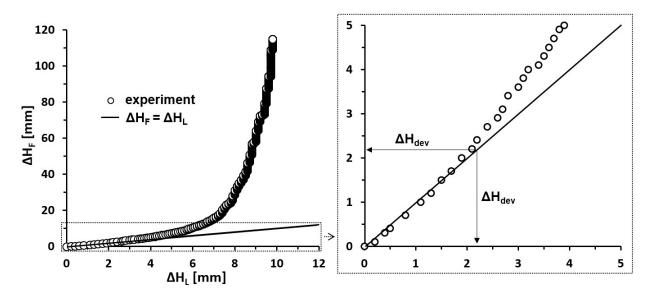
**Figure S2.** (**left**)  $\Delta$ H<sub>F</sub> vs.  $\Delta$ H<sub>L</sub> plot for foam obtained from 100  $\mu$ M BLG solution at pH 3 and C<sub>buff</sub> = 10 mM; a linear regression  $\Delta$ H<sub>F</sub> =  $\Delta$ H<sub>L</sub> is shown for comparison. (**right**) Zoomed-in fragment of the main graph; the common value of  $\Delta$ H<sub>dev</sub> is that measured at t<sub>dev</sub>.
