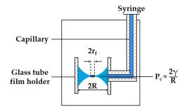
Figure S5. Schematic drawing of the Scheludko-Exerowa tube cell (rf is film radius).
