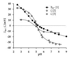
**Figure S1.** Average number of bound protons  $\mathbb{Z}_{H^+}$  (adapted from [1]) and zeta potential  $\zeta$  (adapted from Refs. [2,3]) for BLG solutions as a function of pH; ( $\Diamond$ ) pH adjusted by HCl/NaOH, ( $\Box$ ) McIlvaine buffer (10 mM citric acid + 20 mM Na<sub>2</sub>HPO<sub>4</sub>).
