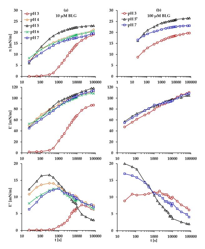
**Figure S8.** Kinetic dependencies of the surface pressure  $\pi(t)$  and the elastic E'(t) and viscous E"(t) parts of the dilational viscoelastic modulus for BLG adsorption layers at the surface of a static air bubble as measured by Profile Analysis Tensiometry; taken from the data sets reported in [7,12]. \* pH 5, C<sub>BLG</sub> = 20 µM.
