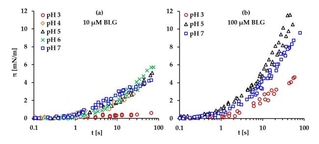
**Figure S7.** Dynamic surface pressure  $\pi(t)$  for BLG adsorption at the surface of a growing air bubble as measured by Bubble Pressure tensiometry.
