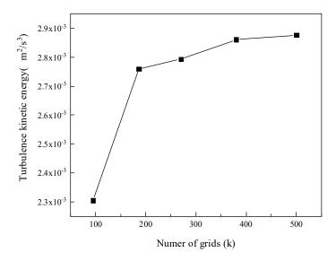
Figure S3. Simulation results obtained using different mesh numbers.
