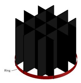
**Figure S2.** Schematic of the media packed in the flotation column.
