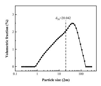
Figure S1. Particle size distribution of the slurry fed to the flotation column.
