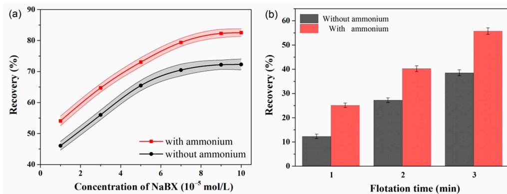
**Figure 1.** (a) Flotation recovery of sulfidized malachite with and without ammonium as a function of NaBX concentration, the flotation time was 10 min. (b) Flotation recovery of sulfidized malachite with and without ammonium as a function of flotation time.  $C(\text{Na}_2\text{S}) = 5 \times 10^{-4}$  M,  $C(\text{NH}_4^+) = 10^{-3}$  M,  $C(\text{NaBX}) = 1 \times 10^{-4}$  M,  $\text{pH} = 10.0 \pm 0.05$ .
