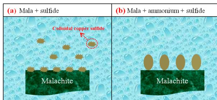
**Figure 11.** Schematic of sulfidization products grown on malachite without (a) and with (b) ammonium ions. The brown floccules and elliptical plates represent the sulfidization products without and with ammonium, respectively.
