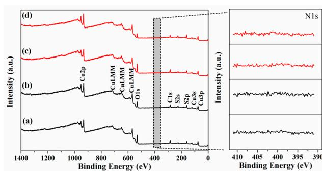
**Figure 8.** XPS survey spectra (left) and corresponding high-resolution N1s spectra (right) of malachite treated with (a)  $5 \times 10^{-4}$  M  $\text{Na}_2\text{S}$  alone, (b)  $3 \times 10^{-3}$  M  $\text{Na}_2\text{S}$  alone, (c)  $5 \times 10^{-4}$  M  $\text{Na}_2\text{S}$  and  $1 \times 10^{-3}$  M  $\text{NH}_4^+$ , (d)  $3 \times 10^{-3}$  M  $\text{Na}_2\text{S}$  and  $6 \times 10^{-3}$  M  $\text{NH}_4^+$ .
