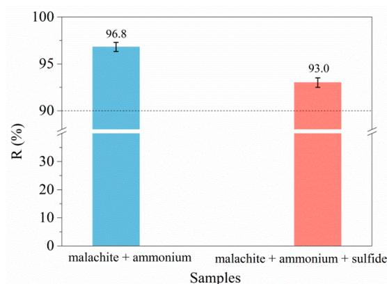
**Figure 10.** Residual ratio of ammonium nitrogen in solution for malachite suspension treated with ammonium solution (malachite + ammonium), or with ammonium and sulfide solution in sequence (malachite + ammonium + sulfide).
