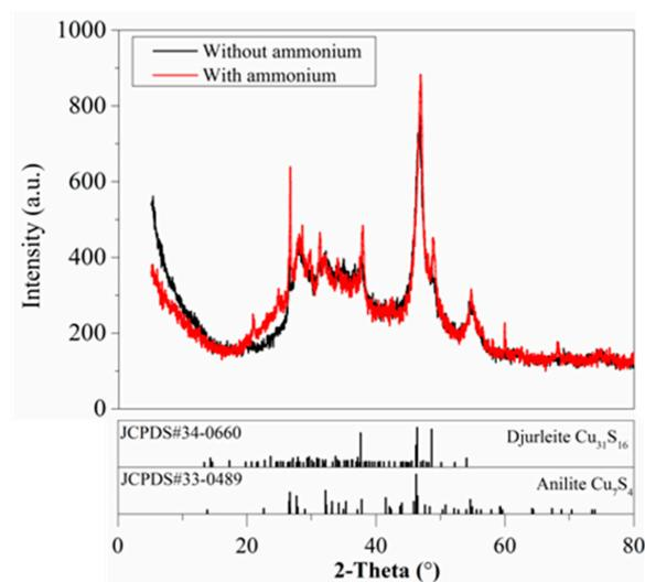
**Figure 6.** XRD patterns of sulfidization products without and with ammonium.  $C(\text{Na}_2\text{S}) = 5 \times 10^{-4}$  M,  $C(\text{NH}_4^+) = 1 \times 10^{-3}$  M.
