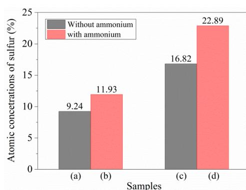
**Figure 9.** Atomic concentration of sulfur at the sulfidized malachite's surface treated with (a)  $5 \times 10^{-4}$  M  $\text{Na}_2\text{S}$ , (b)  $5 \times 10^{-4}$  M  $\text{Na}_2\text{S}$  and  $1 \times 10^{-3}$  M  $\text{NH}_4^+$ , (c)  $3 \times 10^{-3}$  M  $\text{Na}_2\text{S}$ , and (d)  $3 \times 10^{-3}$  M  $\text{Na}_2\text{S}$  and  $6 \times 10^{-3}$  M  $\text{NH}_4^+$ .
