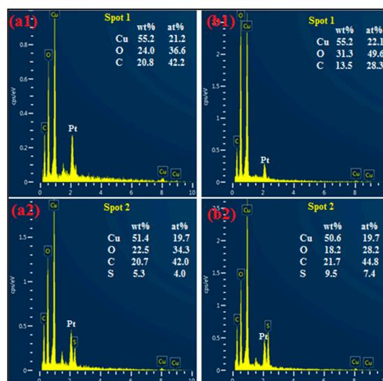
**Figure 4.** EDS results for sulfidized malachite produced (a1,a2) without of ammonium and (b1,b2) with ammonium, corresponding to Figure 3a,b, respectively.
