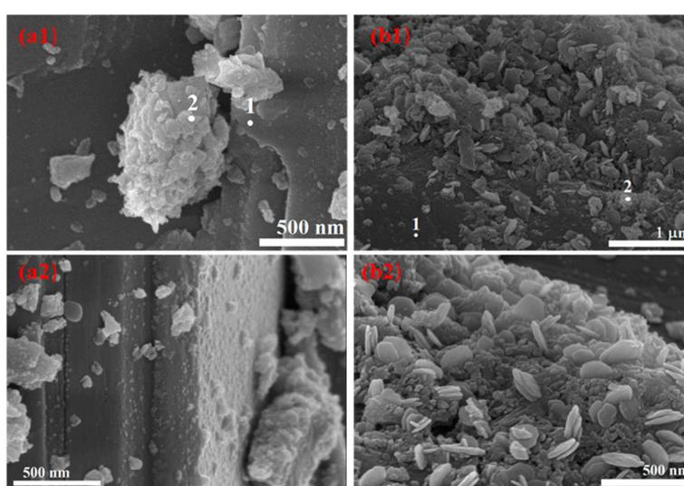
**Figure 3.** FESEM images of sulfidized malachite (a1,a2) without ammonium ions and (b1,b2) with ammonium ions.  $C(\text{Na}_2\text{S}) = 5 \times 10^{-4}$  M,  $C(\text{NH}_4^+) = 10^{-3}$  M.
