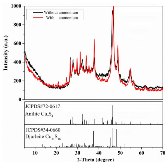
**Figure 7.** XRD patterns of sulfidization products without and with ammonium.  $C(\text{Na}_2\text{S}) = 3 \times 10^{-3}$  M,  $C(\text{NH}_4^+) = 6 \times 10^{-3}$  M.
