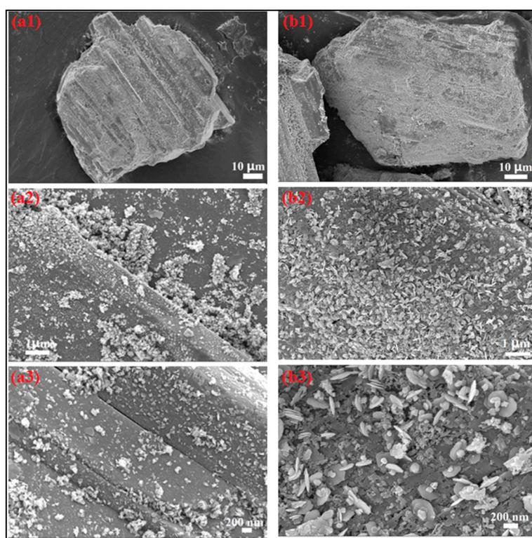
**Figure 5.** FESEM images of sulfidized malachite (a1,a2,a3) without ammonium and (b1,b2,b3) with ammonium.  $C(\text{Na}_2\text{S}) = 3 \times 10^{-3}$  M,  $C(\text{NH}_4^+) = 6 \times 10^{-3}$  M.
