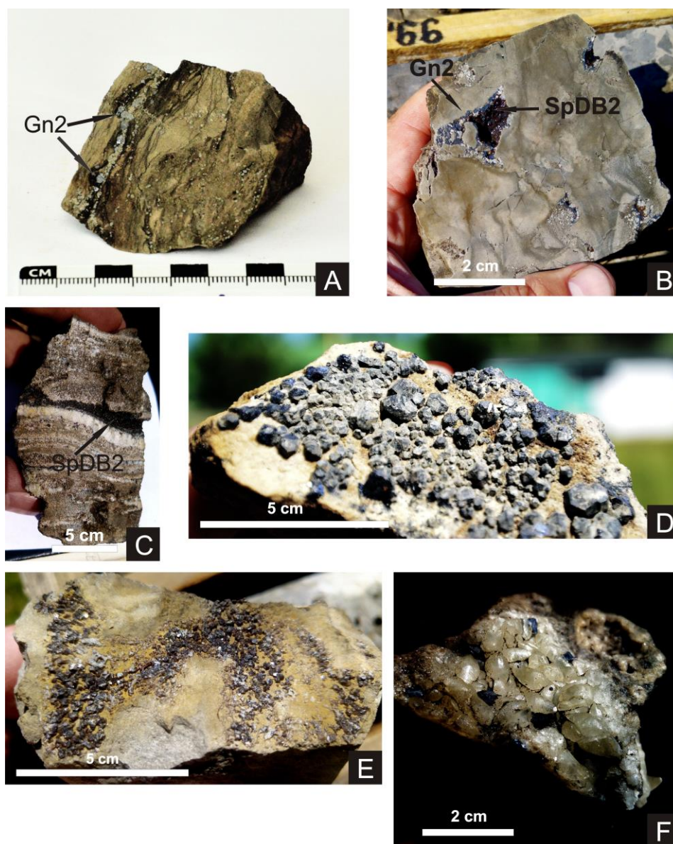
Figure 13. (A) Galena (Gn2) crystals within irregularly streaked dolomite, Zawiercie 93 TN borehole; (B) dolomite with visible unstable density layering structures, with many caverns partly filled with sphalerite and galena, Zawiercie TN 87 borehole; (C) stratified Zn-Pb ore, “zebra-type”, Poręba MZ 23 borehole; (D) well-formed galena, in form of octahedrons and cubes, Gołuchowice 21 G borehole; (E) sphalerite crystallized on the cracked dolomite surface, Gołuchowice 2 G borehole; and (F) galena and white calcite forming the matrix of hydrothermal breccia, Kierszula TN 245 borehole.
