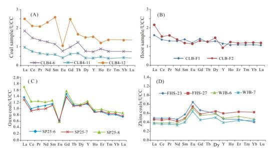
**Figure 13.** Distribution patterns of rare earth elements and yttrium (REY) in the study coals (**A**), floor rocks (**B**), Guxu coals (**C**) [21], and Zhina coals (**D**) [12]. REY are normalized to Upper Continental Crust [55].
