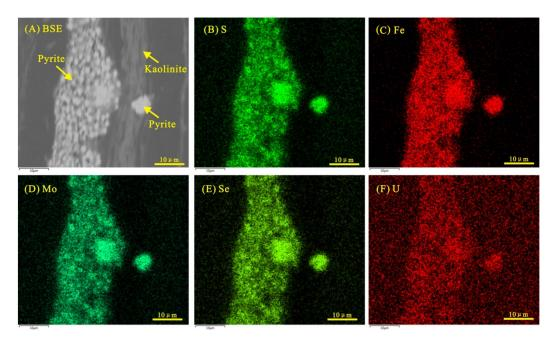
**Figure 12.** SEM-EDS mapping showing the distribution of S, Fe, Mo, Se, and U (sample CLB4-1). **(A)**: SEM back-scattered electron images of minerals; **(B)**–**(F)**: the distribution of S, Fe, Mo, Se, and U, respectively.
