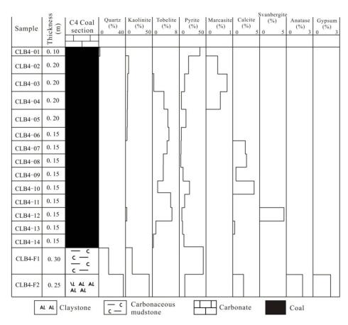
Figure 3. Vertical distribution of the minerals identified in the C4 Coal (on whole-coal basis).
