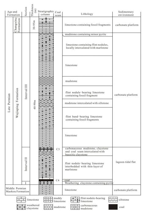
**Figure 2.** Sedimentary sequence of the Late Permian Wujiaping Formation in the Tongzi Coalfield (Based on the exploration data from Guizhou Province Geology and Mineral Bureau).
