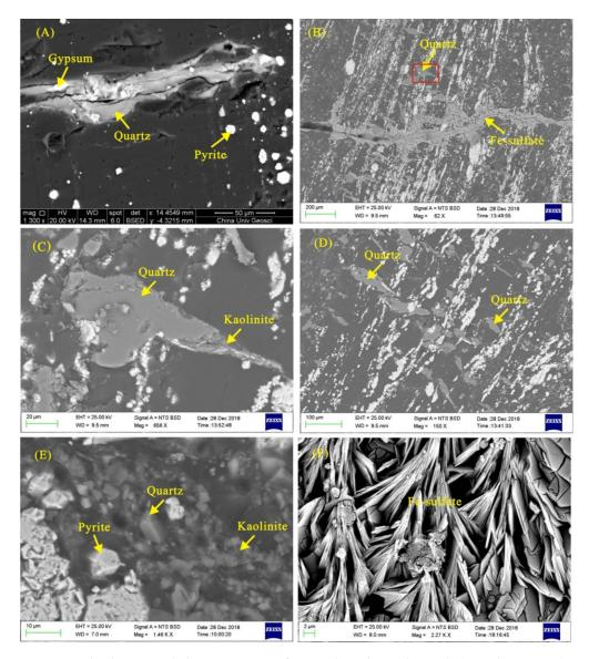
**Figure 9.** SEM back-scattered electron images of minerals in the coal sample (sample CLB4-12) and floor sample (sample CLB4-F1). (**A**): fracture-filling quartz and gypsum; (**B**): fracture-filling quartz and Fe-sulfate; (**C**): fracture-filling quartz, with kaolinite occurring along the outer edge of quartz; (**D**): fracture-filling quartz; (**E**): kaolinite matrix, dispersed pyrite particle, and euhedral quartz grain; (**F**): needle-like Fe-sulfate.
