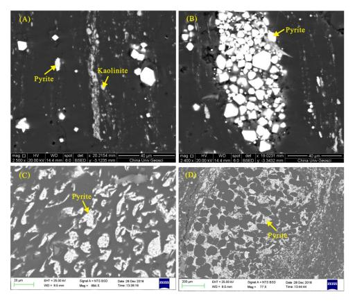
**Figure 6.** Scanning electron microscope (SEM) back-scattered electron images of minerals in the C4 Coal. (**A**): isolated pyrite and kaolinite grains (sample CLB4-12); (**B**): euhedral pyrite aggregate (sample CLB4-12); (**C**) and (**D**): cell-filling pyrite (sample CLB4-2).
