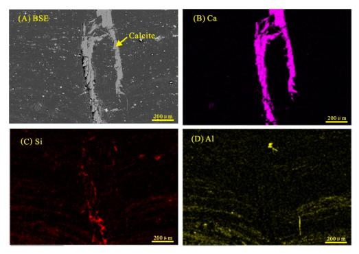
**Figure 10.** SEM-EDS mapping showing the distribution of Ca, Si, and Al (sample CLB4-7). (**A**): SEM back-scattered electron images of minerals; (**B**)–(**D**): the distribution of Ca, Si, and Al, respectively.
