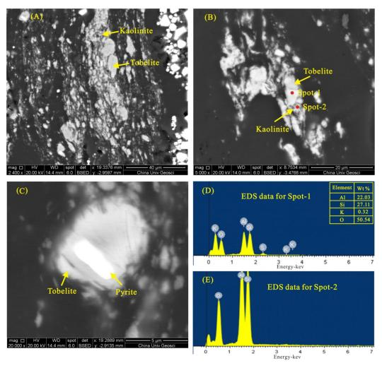
**Figure 8.** SEM back-scattered electron images of minerals in the coal sample (sample CLB4-12) and EDS analysis of selected minerals. (**A**): dispersed kaolinite and tobelite particles along bedding planes; (**B**): pore space-filling tobelite; (**C**): pore space-filling tobelite containing an inclusion of pyrite; (**D**): EDS spectra of tobelite containing trace K; (**E**): EDS spectra of kaolinite.
