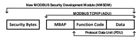
Figure 7. New MODBUS Security Development Module.
