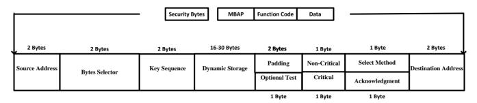
Figure 8. Cryptography Buffer (CB) Fields.
