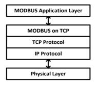
Figure 2. MODBUS Protocol Stack with an Internet Protocol Suite.
