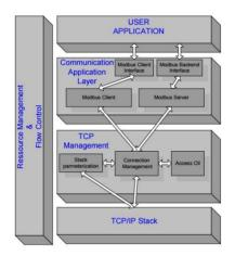
Figure 6. MODBUS Messaging Architecture and TCP/IP Stack [5].
