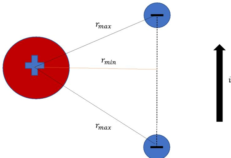
Figure 5. Two electrons from a train of electrons, moving in the vicinity of a proton.
