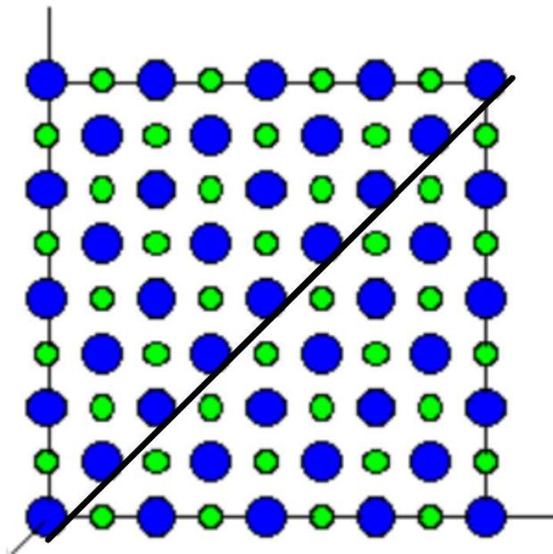
**Figure 7.** The 100 planes of a lattice of  $Na^+Cl^-$  (table salt): blue circles depict sodium positive ions, and green circles depict chlorine negative ions. The trajectory of relativistic electrons is described using a thick black line.
