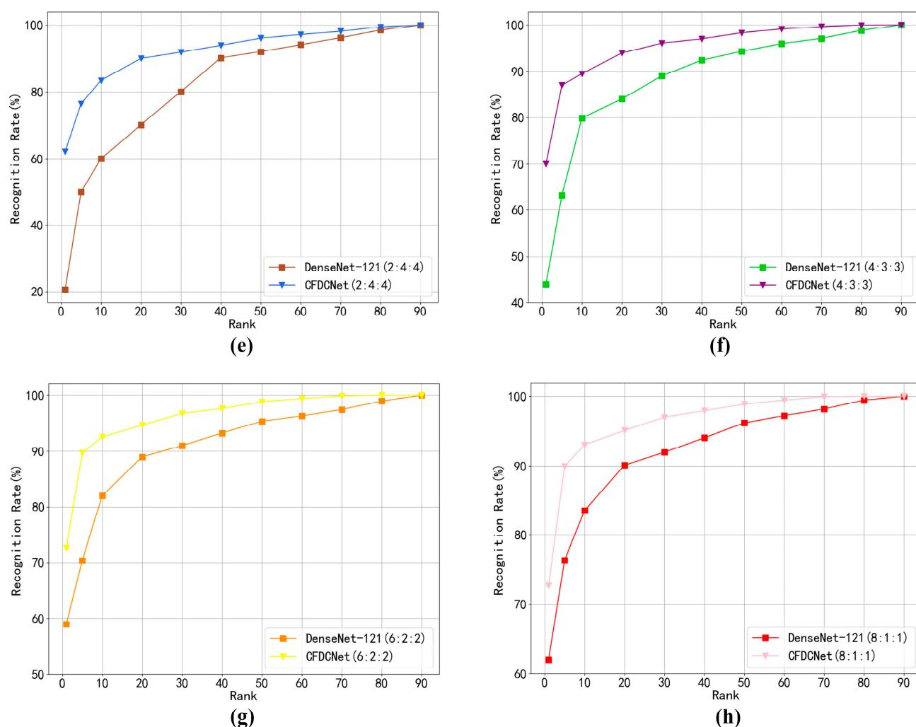
**Figure 12.** The CMC curves compare the recognition performance of DenseNet-121 and CFDCNet with different dataset division ratios. Where (a–d) are the CMC curves for the AMI dataset with different division ratios, and (e–h) are the CMC curves for the AWE dataset with different division ratios.
