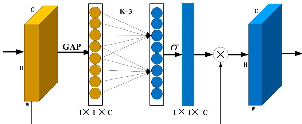
**Figure 6.** Efficient Channel Attention (ECA) module structure diagram.
