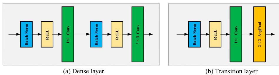
**Figure 4.** Structure diagram of the Dense layer and Transition layer before improvement.
