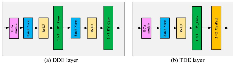
**Figure 3.** Structure diagram of the DDE layer and the TDE layer.
