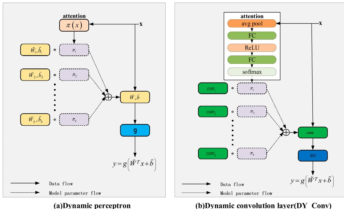
**Figure 5.** Structure diagram of a dynamic perceptron and a dynamic convolution layer (DY\_Conv). The asterisk represents multiplication.
