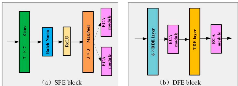
**Figure 2.** Schematic diagram of the SFE block and the first DFE block structure.
