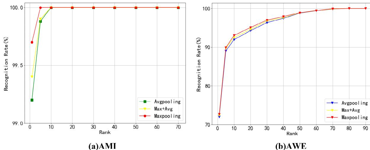
**Figure 11.** The CMC curves compare the recognition performance under different pooling methods.
