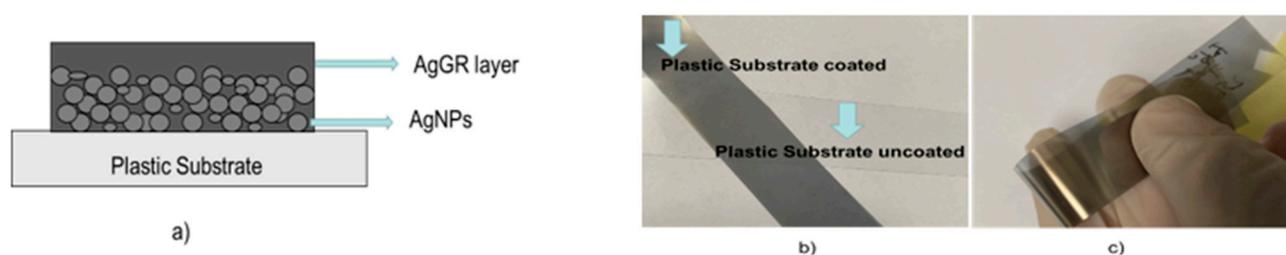
**Figure 1.** The design of the electrochemical sensor is based on: (a) the AgGR nanocomposite layer and AgNPs, (b) a digital photo of the coated and uncoated plastic substrate, and (c) flexibility of the sample.
