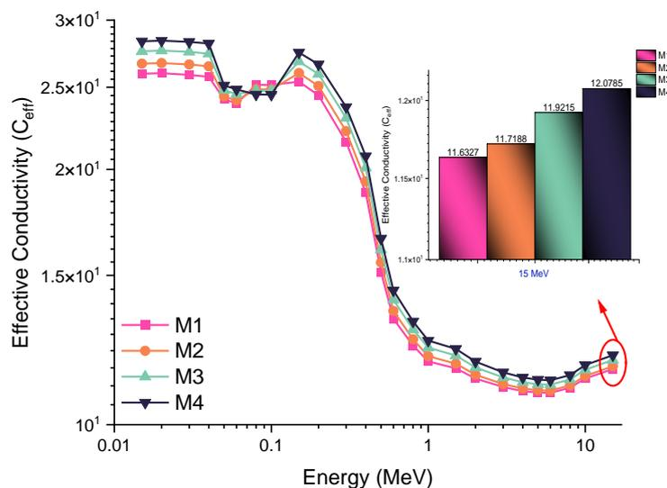
**Figure 7.** Variation of effective conductivity ( $C_{\text{eff}}$ ) with photon energy (MeV) for all M1–M4 glasses.
