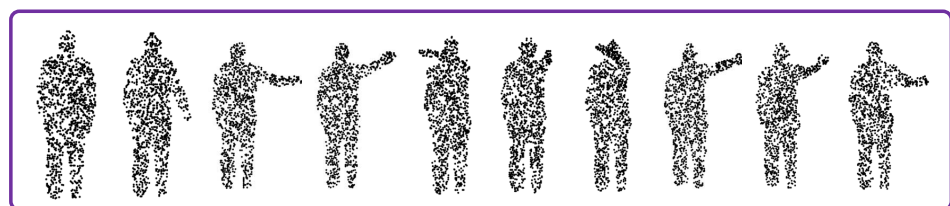
Figure 4. The point cloud sequence of horizontal arm wave in the MSR Action3D dataset.
