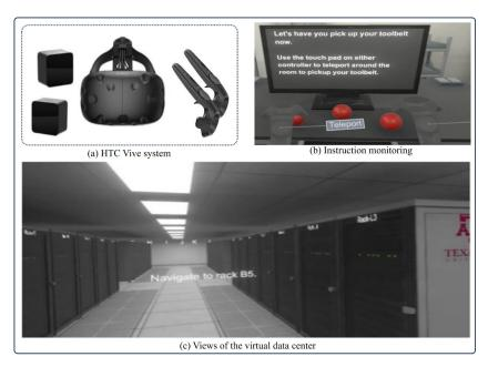
**Figure 2.** CiSE-ProS: [75] (**a**) The HTC Vive system, including headsets, motion trackers, and handheld controllers. (**b**) The tutorial room had an instruction monitor. (**c**) Views of the virtual data center.
