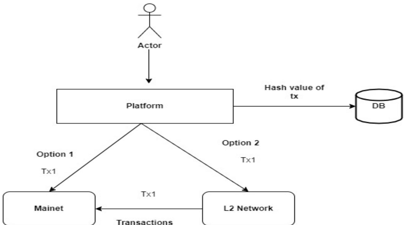
**Figure 1.** A Revised L2 Solution on DpoS.
