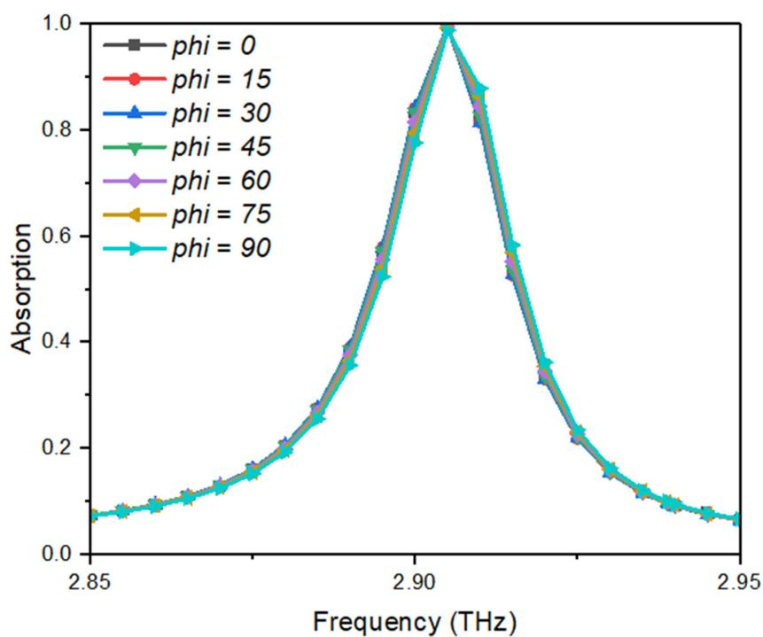
**Figure 6.** Absorption spectrum for different polarization angles.
