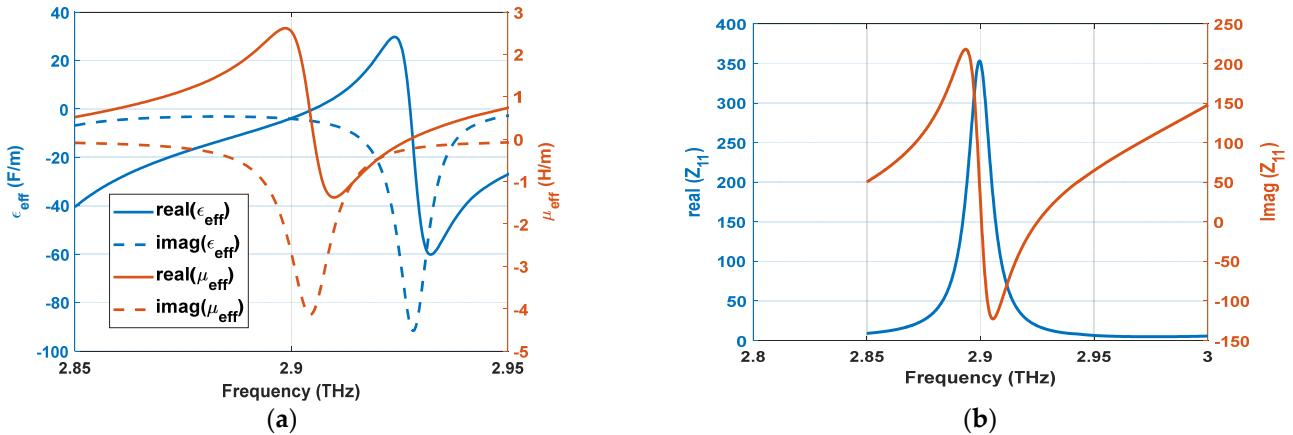
**Figure 4.** (a) Effective permittivity and permeability of the proposed design (b) Impedance characteristics of the design.
