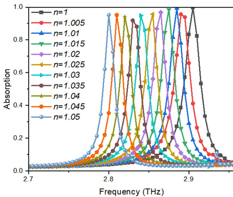
**Figure 7.** Absorption Spectrum for different refractive indices at the resonant frequency.
