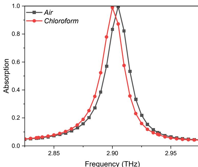
**Figure 9.** Absorption spectrum for refractive index of chloroform at resonant frequency.
