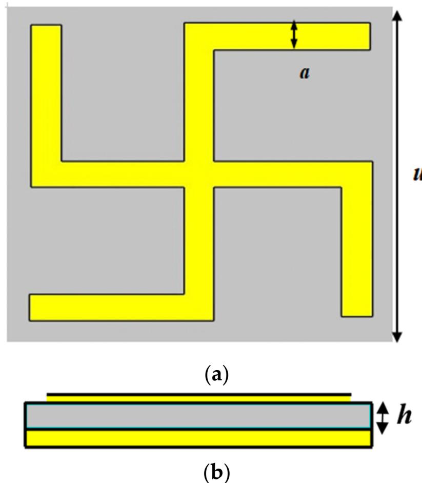
**Figure 1.** Proposed structure of terahertz metamaterial absorber: (a) top view; (b) side view.
