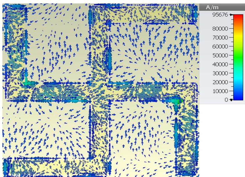
**Figure 3.** Surface current distribution at the resonant frequency.
