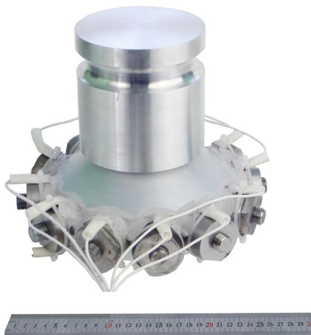
**Figure 3.** Transducer assembled with a cylindrical radiator.
