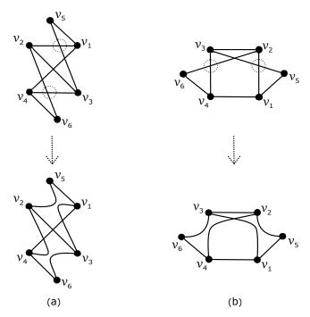
**Figure 3.** Elimination of two crossings on edges of  $G^*$  with vertex notation in a different order for both bottom drawings, after which, edges of  $C_4(G^*)$  cross each other. (a): elimination of two crossings on edges of  $C_4(G^*)$  with  $\operatorname{cr}_D(G^*) = 5$ ; (b): elimination two crossings on edges of  $C_4(G^*)$ with  $\operatorname{cr}_D(G^*) = 3$ .
