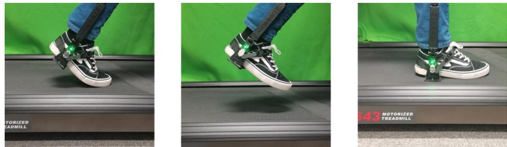
**Figure 2.** Relationship between the foot and ground of the lower limb exoskeleton robot: foot lift (L), foot hang (H), and foot support (S).
