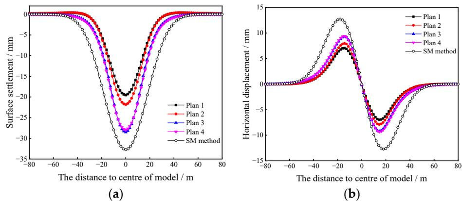
**Figure 18.** Surface Displacement Curves Caused by pilot tunnel excavation: (a) surface settlement, and (b) surface horizontal displacement.
