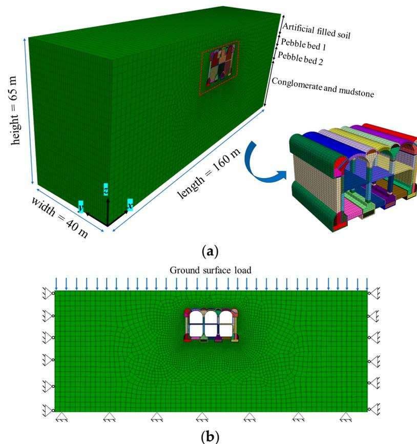
**Figure 3.** Numerical model: (a) Finite element mesh; (b) Boundary conditions.
