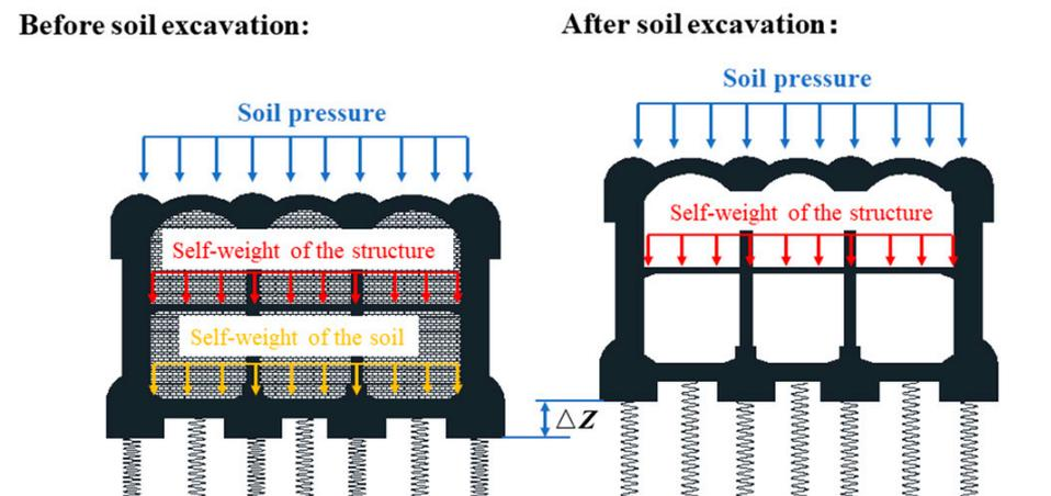
Figure 8. Strata displacement rebound mechanism.
