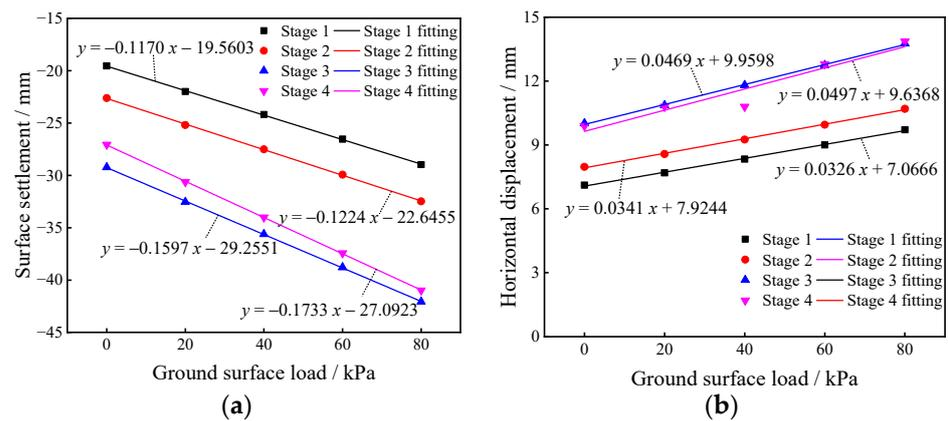
Figure 12. Fitting curves of surface displacement under different loads: (a) surface settlement; and (b) surface horizontal displacement.
