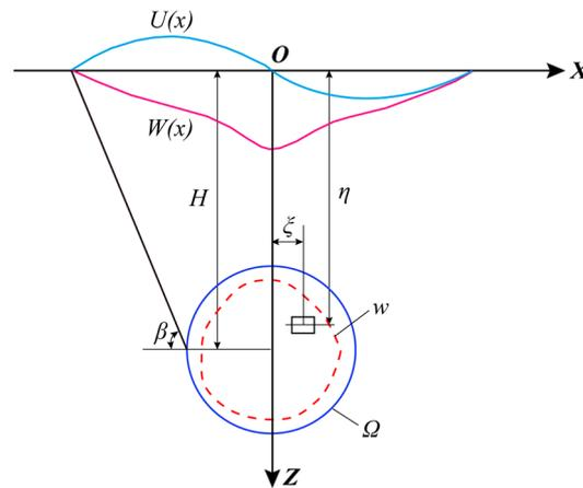
Figure 16. Analysis of ground deformation and section shrinkage in tunnel excavation.
