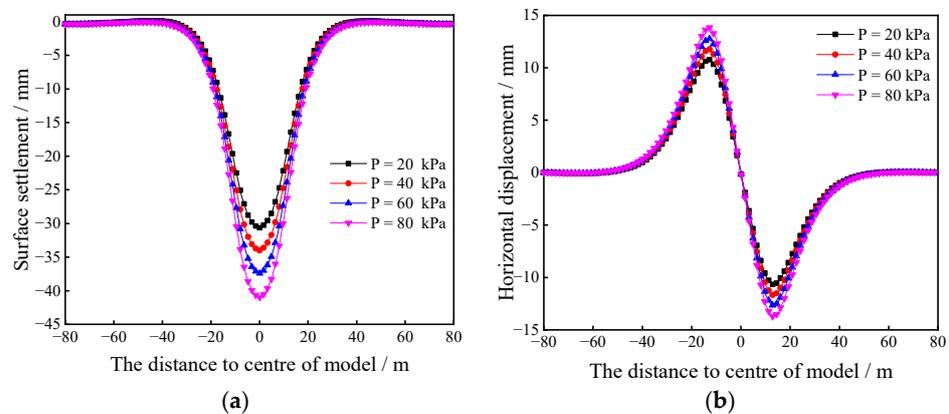
Figure 11. Surface displacement curves under different loads: (a) surface settlement; and (b) surface horizontal displacement.
