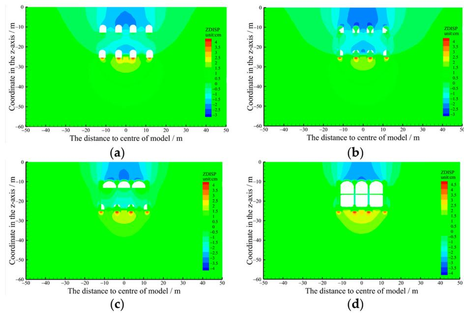
**Figure 6.** Vertical displacement of strata in different stages: (a) Stage I; (b) Stage II; (c) Stage III; and (d) Stage IV.
