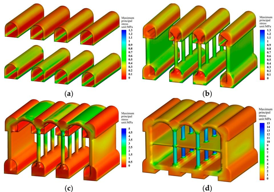
**Figure 9.** The maximum principal stress distribution of structure in different stages: (a) Stage I; (b) Stage II (c); Stage III; and (d) Stage IV.
