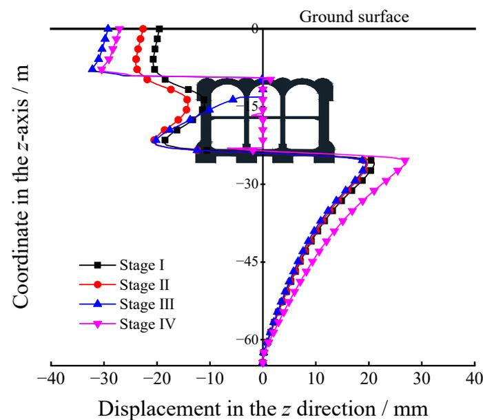
**Figure 7.** Vertical displacement of model center in different stages.
