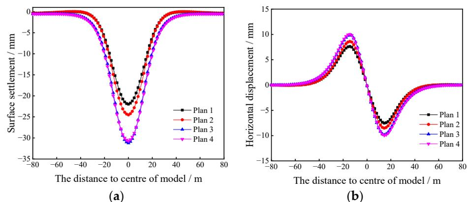
**Figure 15.** Surface displacement curves in different plans: (a) surface settlement; and (b) surface horizontal displacement.
