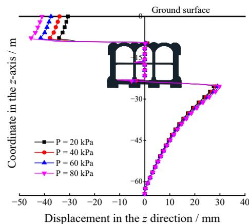
**Figure 13.** Vertical displacement of the model center under different loads.
