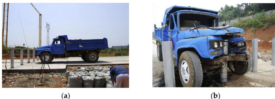
**Figure 4.** Full-scale truck crash test: (a) before and (b) after the collision [14]. (Reprinted with permission from Ref. [14]. 2015, Elsevier.)
