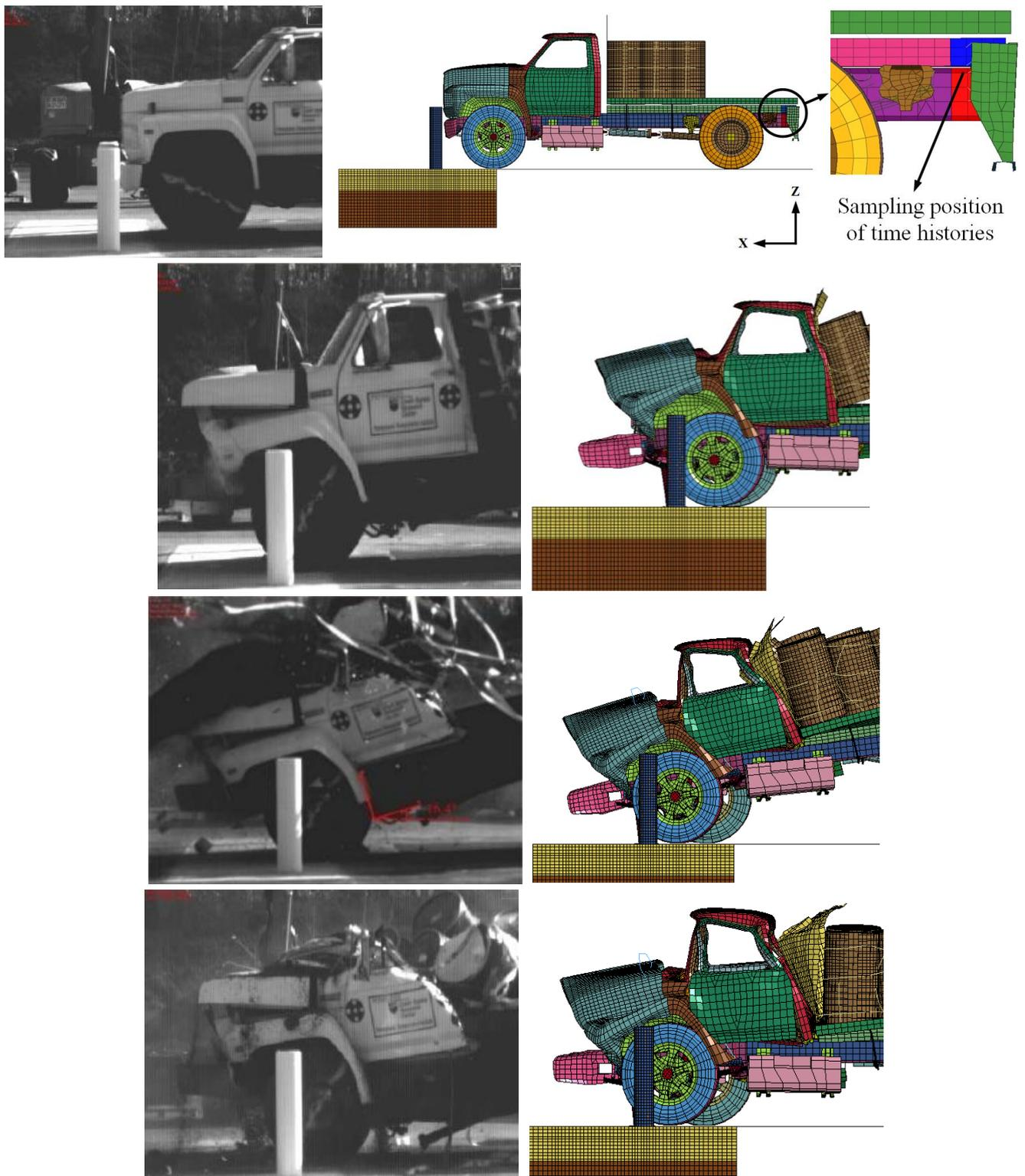
Figure 9. Comparison of the collision process between Test I and the simulation.
