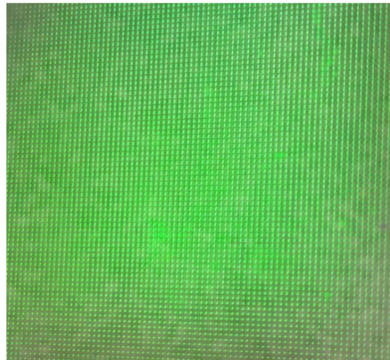
Figure 6. Reconstruction of the lens array using the LAHOE with Bragg matched light.
