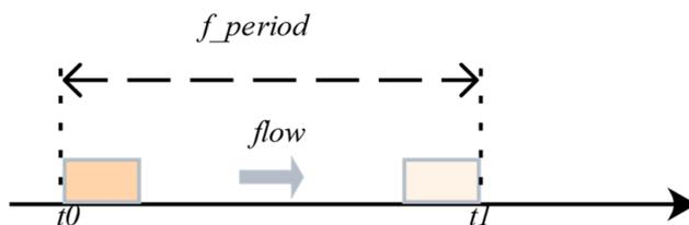
Figure 4. Flow should be constrained to be transmitted within the period.
