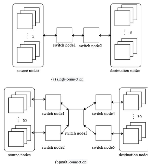
**Figure 12.** Network topology models of scales 10 and 100 (a) single connection; (b) multi connection.
