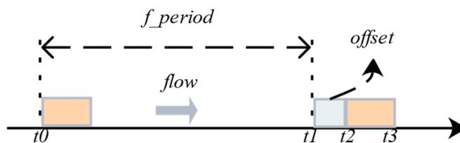
Figure 5. Under the effect of the offset, the transmission of the flow.
