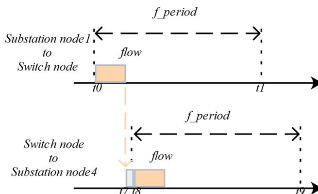
Figure 7. When there is an offset, the transmission period is constrained.
