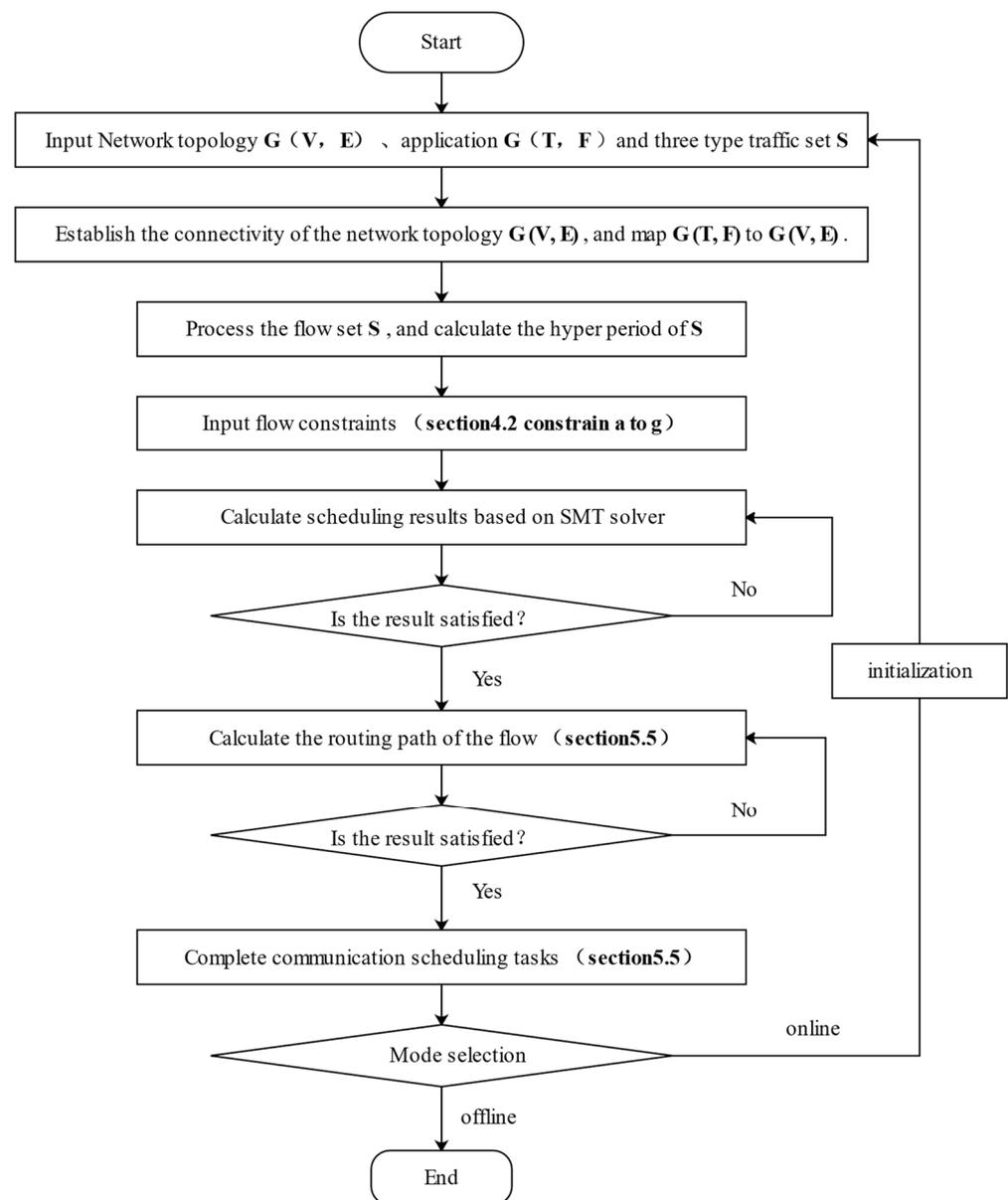
**Figure 10.** Overall process chart of the routing and scheduling algorithm.
