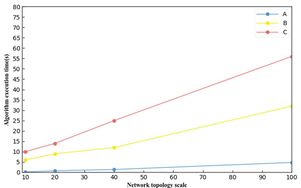
Figure 14. Impact of network topology scale on algorithm execution time.
