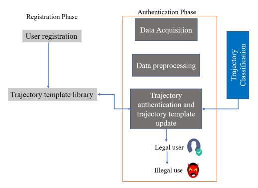
Figure 3. Architecture of system for trip trajectory authentication.
