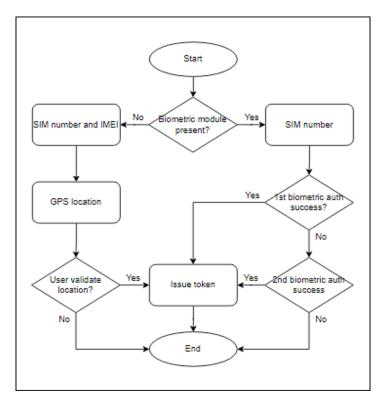
Figure 8. Biometric-geo mobile identity authentication.
