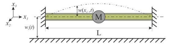
Figure 7. Kinematic scheme of loading of flexoelectric beam with proof mass M.
