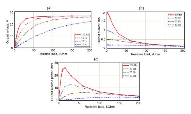
**Figure 35.** Dependencies of the output voltage (**a**), current (**b**), and generated output power (**c**) on the excitation frequency f and electric load resistance R (from Shevtsov et al. [77] reproduced by permission of Springer Nature © 2022).
