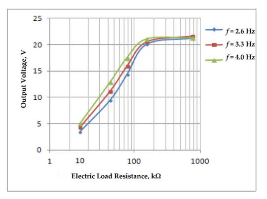
**Figure 32.** Output voltage in dependence on electric load resistance under harmonic excitation to frequency of 4 Hz at mechanical loading with value of 8.8 MPa.
