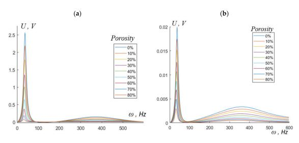
**Figure 19.** Output voltage on the (**a**) bimorph plates, located on the PEG cantilever substrate; (**b**) PEG piezoelectric cylinders vs. the frequency range of harmonic excitation from 0 to 600 Hz.
