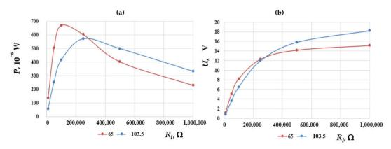
**Figure 15.** Output power (**a**) and output voltage (**b**) vs. active load for two locations of proof mass:  $L_m = 65$  and 103.5 mm.
