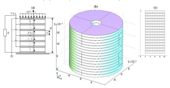
**Figure 34.** FE model of stack-type PEG under homogeneously distributed mechanical load: (**a**) common scheme, (**b**) an example of modeled stack geometry, and (**c**) FE partition of axisymmetric model (from Shevtsov et al. [77], reproduced by permission of Springer Nature © 2022).
