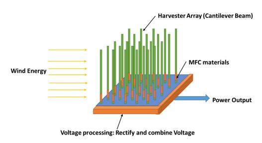
**Figure 25.** Energy harvesters from artificial grass (from Haldkar et al. [235], reproduced by permission of Springer Nature © 2022).
