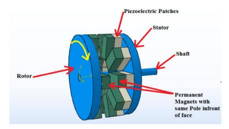
**Figure 1.** Configuration of piezoelectric energy harvester with parallel coaxial plates (from Narolia et al. [178], reproduced by permission of Springer Nature © 2022).
