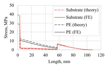
Figure 21. Stress distribution in cantilever PEG along its length on the upper surfaces of layers.
