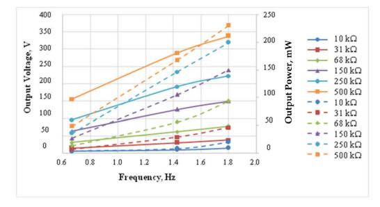
**Figure 30.** Output voltage (continuous curve) and output power (dotted curve) in dependence on impact frequency at various values of load resistance for the ring-type PEG with a thickness of 38 mm at a pulse mechanical load of 17.2 MPa.
