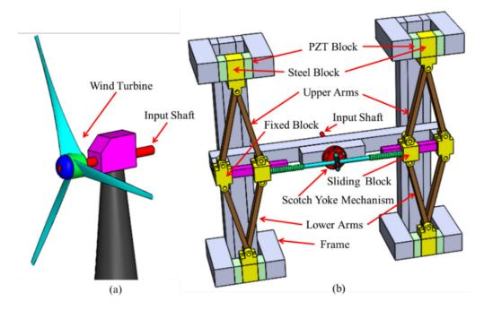
**Figure 3.** (a) Configuration of wind turbine and (b) energy harvester with scissor mechanism (from Narolia et al. [180], reproduced by permission of Springer Nature © 2022).
