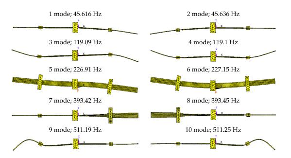
Figure 24. First ten modes of the eigen-forms of PEG with symmetric fixing of load oscillations.
