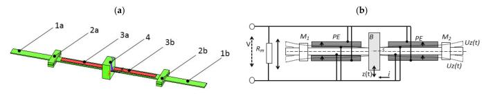
**Figure 23.** (**a**) Biaxial PEG model with symmetrically-located proof masses; (**b**) electric scheme of PEG under active load.
