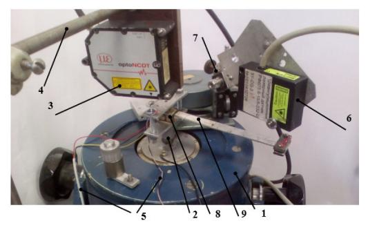
**Figure 10.** Vibration setup with PEG: 1—vibrating table; 2—PEG; 3—laser sensor optoNSDT of displacement; 4—support of laser sensor 3; 5—electric path of PEG; 6—triangulation laser sensor of displacements RF603; 7—sensor support stand (6); 8—cylindrical PEs, located at the base of the PEG; and 9—PE plates.
