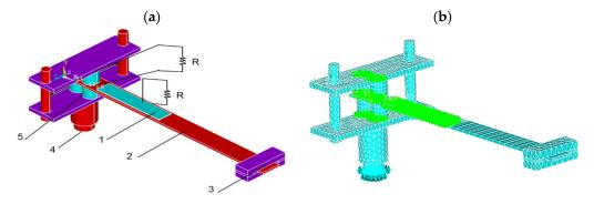
Figure 18. (a) Location of electrical load on model; and (b) FE-scheme of PEG with proof mass.
