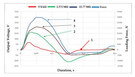
**Figure 29.** Shapes of piezoelectric output voltage (1–3) and pulses of compression force (4) in dependence on electric load resistance.
