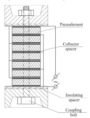
Figure 26. Stack-type converter.
