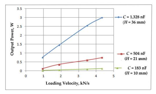
**Figure 31.** Peak output power vs. PEG quasi-static loading velocity at various stack heights and electrical capacitance.
