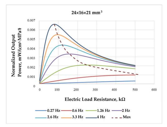
**Figure 33.** Normalized output power in dependence on electric load resistance under harmonic excitation at various frequencies from 0.27 to 4 Hz.
