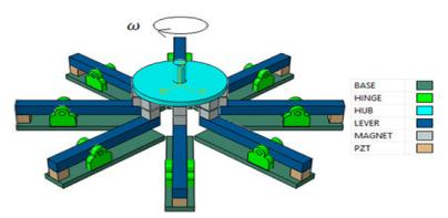
**Figure 2.** Configuration of energy harvester with rotating hub (from Narolia et al. [179], reproduced by permission of Springer Nature © 2022).
