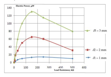
**Figure 12.** Dependence of output electric power on load resistance for various values of displacement amplitude of free tip of the cantilever at a proof mass of 20.6 g.
