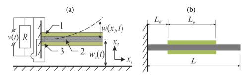
**Figure 20.** (a) Bimorph cantilever PEG: 1 and 3—piezoelements, 2—substrate; (b) cantilever-type PEG with incomplete piezoelectric coating of the substrate.
