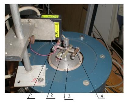
**Figure 13.** Experimental set-up for research of double-cantilever PEG: the numbers point out displacement measurer (1), accelerometer (2), shaker (3), and proof mass (4).
