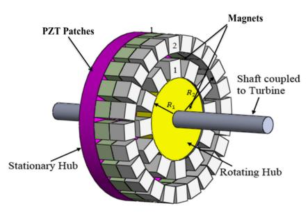
**Figure 4.** Configuration of energy harvester (from Narolia et al. [181], reproduced by permission of Journal of Advanced Dielectrics, Vol. 10, No. 03, @ 2020 and World Scientific Publishing Co. Pte. Ltd.).
