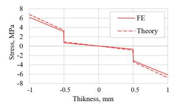
Figure 22. Stress distribution in cantilever PEG over thickness in the middle part of piezoelement.
