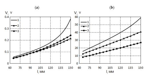
**Figure 17.** Dependencies of voltage amplitude: (**a**) for the first model; (**a**) for the second model: 1—fiberglass; 2—duralumin; and 3—steel.
