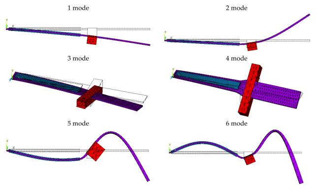
Figure 16. First six modes of vibration eigen-forms for asymmetrical disposition of proof mass.
