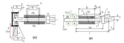
**Figure 9.** (a) Electrical scheme of PEG at vibration loading and (b) structural scheme of PEG with proof mass: 1—plate piezoelectric elements (PEs); 2—substrate; 3—proof mass; 4—PEG fixation point (with movable base *b*); and 5—cylindrical PE.
