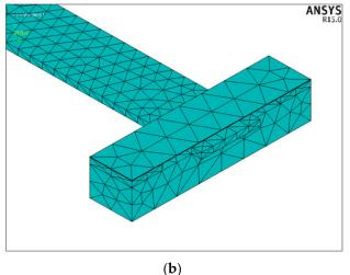
Figure 14. (a) Symmetrical and (b) asymmetrical arrangement of proof mass.
