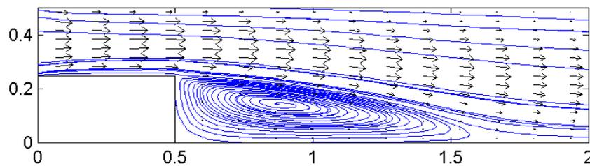
Figure 5. The uncontrolled fluid flow.
