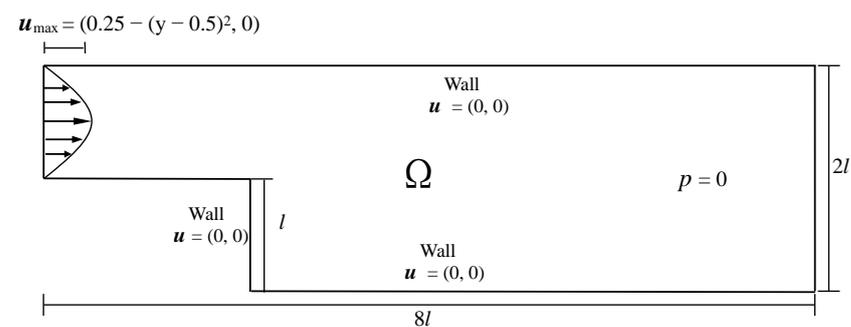
Figure 1. The computational domain of the back-step problem.
