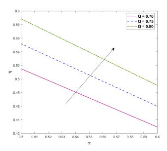
**Figure 9.** Impact of *Q* on fin efficiency.
