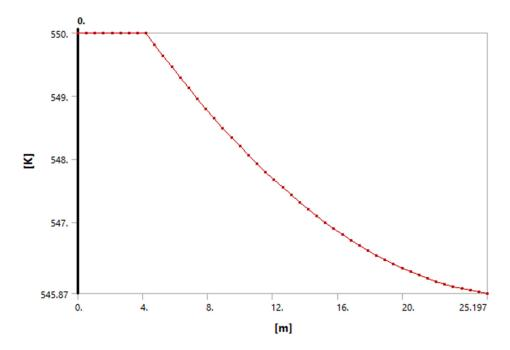
Figure 18. Temperature varying along the length of the fin for Aluminum Alloy 6061.
