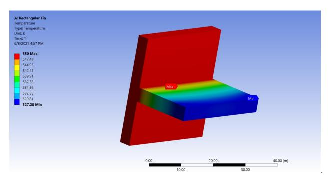
Figure 19. Temperature distribution for Cast Iron.
