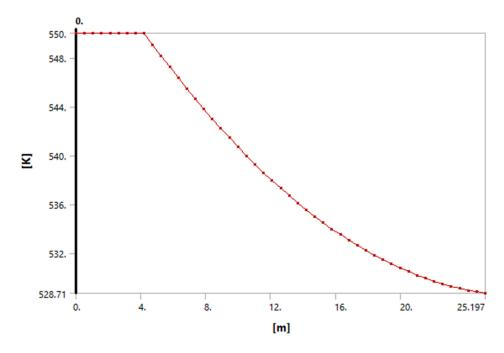
Figure 20. Temperature varying along the length of the fin for Cast Iron.
