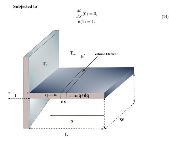
Figure 1. Schematic representation of a longitudinal fin.
