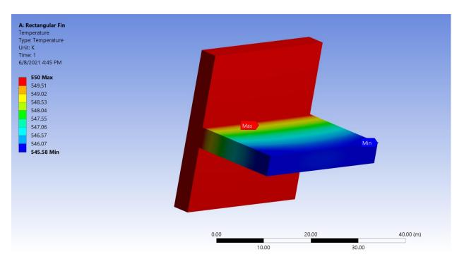
Figure 17. Temperature distribution for Aluminum Alloy 6061.
