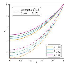
**Figure 16.** Comparing the temperature distribution of a fin with exponential temperature-dependent and linearly temperature-dependent thermal conductivity.
