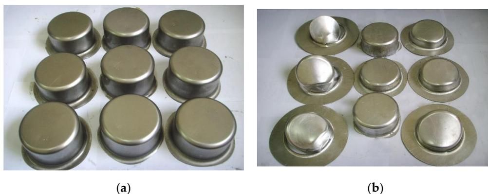
**Figure 13.** Stamping test parts (a) Intact parts; (b) Cracked parts.
