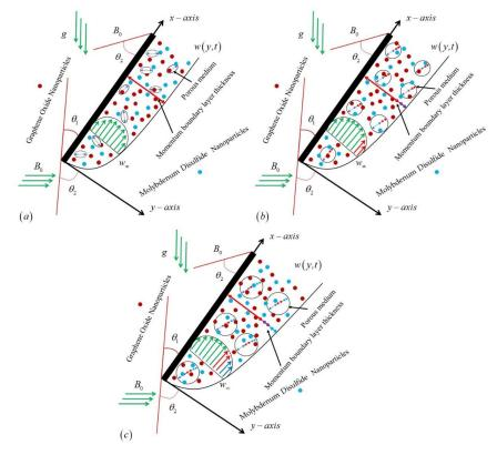
**Figure 13.** Geometrical representation to show the variation of velocity profile in the presence of (a) small porous parameter (b) larger porous parameter and (c) very large porous parameter.
