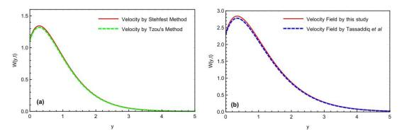
**Figure 12.** Comparison of velocity profile (a) with previously published works for the limiting cases (b) [32].
