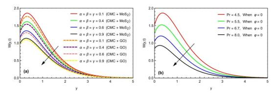
**Figure 5.** Impact of (a)  $\alpha$ ,  $\beta$ ,  $\gamma$  and (b) Pr on momentum profile when M=1.7, Gr=6.3, Gm=6.4, Sc=2.3, b=0.4,  $\omega=0.5$ ,  $\theta_1=\theta_2=\frac{\pi}{4}$ , K=0.5, t=0.8, and  $\varphi=0.2$ .
