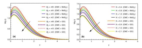
**Figure 8.** Impact of (a)  $\theta_2$  and (b) *K* on momentum profile when  $\alpha = \beta = \gamma = 0.6$ , M = 1.7, Gr = 6.3, Gm = 6.4, Sc = 2.3, b = 0.4,  $\omega = 0.5$ ,  $\theta_1 = \frac{\pi}{4}$ , t = 0.8, and  $\varphi = 0.2$ .
