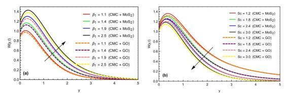
**Figure 9.** Impact of (a)  $\beta_1$  and (b) Sc on momentum profile when  $\alpha = \beta = \gamma = 0.6$ , M = 1.7, Gr = 6.3, Gm = 6.4, b = 0.4,  $\omega = 0.5$ ,  $\theta_1 = \theta_2 = \frac{\pi}{4}$ , K = 0.5, t = 0.8, and  $\varphi = 0.2$ .
