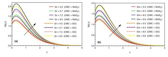
**Figure 6.** Impact of (a) *Gr* and (b) *Gm* on momentum profile when  $\alpha = \beta = \gamma = 0.6$ , M = 1.7, Sc = 2.3, b = 0.4,  $\omega = 0.5$ ,  $\theta_1 = \theta_2 = \frac{\pi}{4}$ , K = 0.5, t = 0.8, and  $\varphi = 0.2$ .
