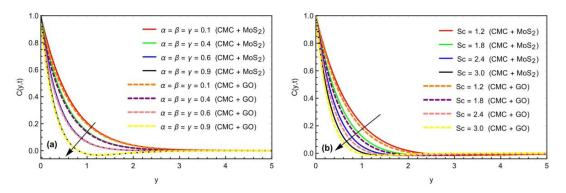
**Figure 4.** Impact of (a)  $\alpha$ ,  $\beta$ ,  $\gamma$ , and (b) Sc on concentration profile when t = 0.8, and  $\varphi = 0.2$ .
