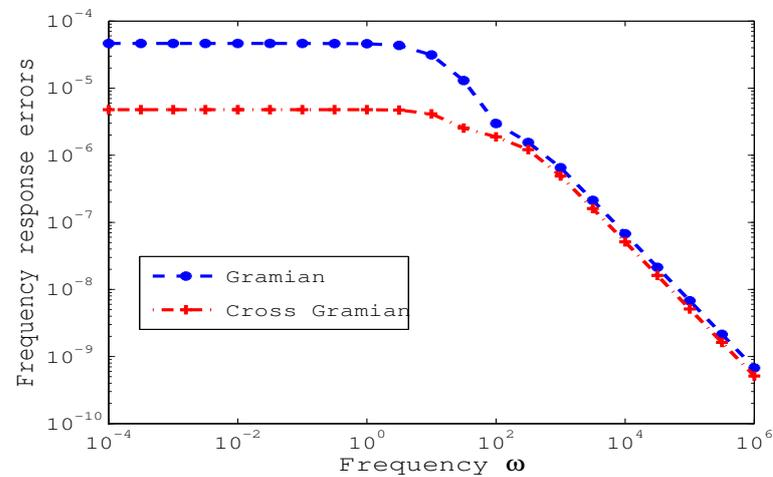
**Figure 3.** The frequency response errors of the MIMO reduced system generated by the Gramian-based BFSR method and the cross-Gramian-based BFSR method with the reduced order  $l = 16$ .
