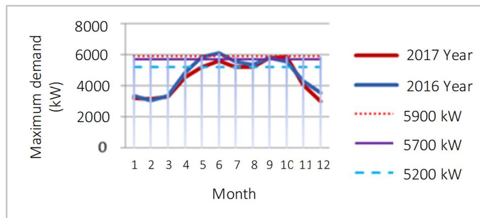
**Figure 3.** The changes in monthly maximum demand in the MOF1 main substation.
