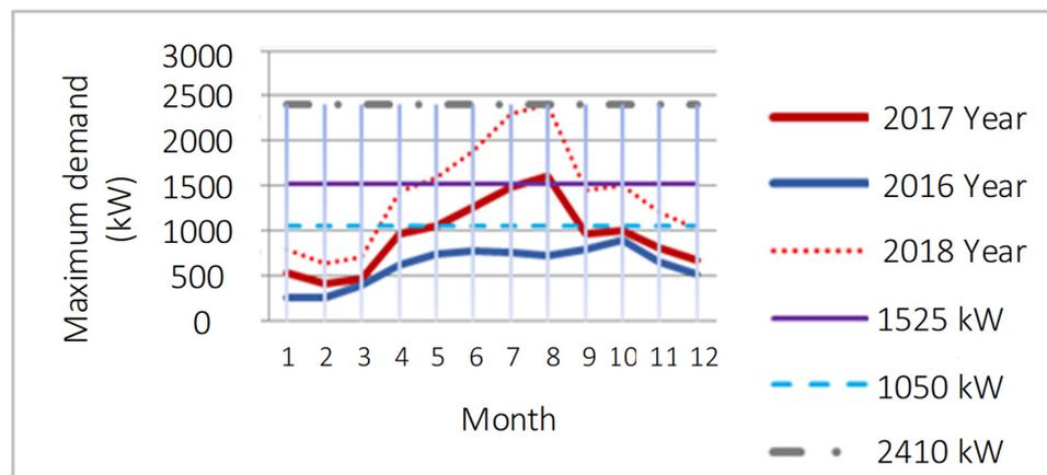
Figure 6. The predicted changes in monthly maximum demand in the MOF3 main substation.
