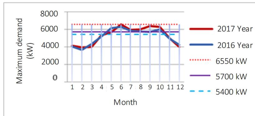
Figure 4. The changes in monthly maximum demand in the MOF2 main substation.
