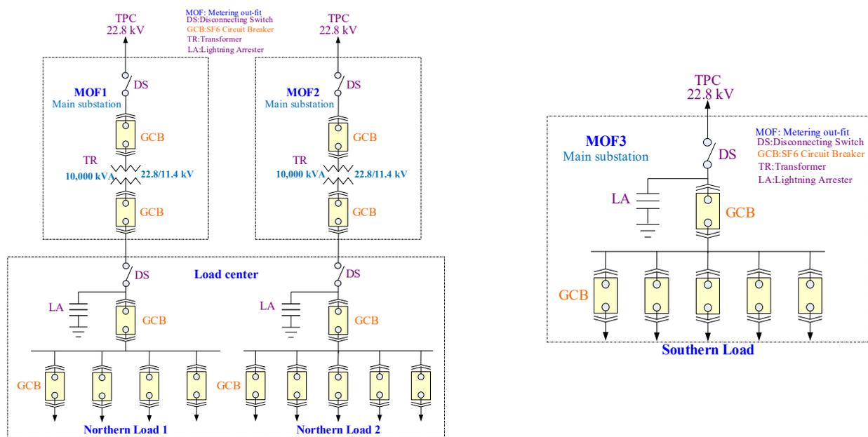
Figure 2. The single diagram of a power system in a famous university.
