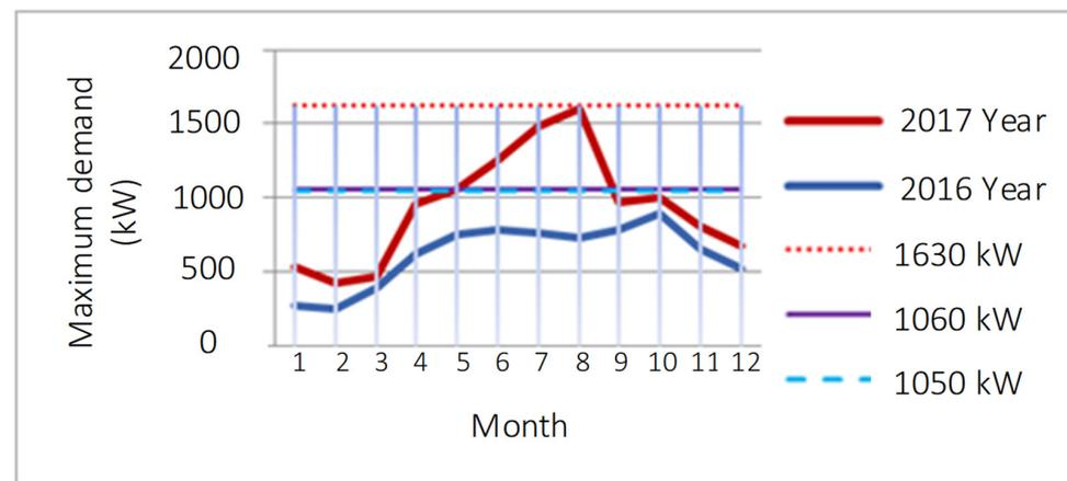
**Figure 5.** The changes in monthly maximum demand in the MOF3 main substation.
