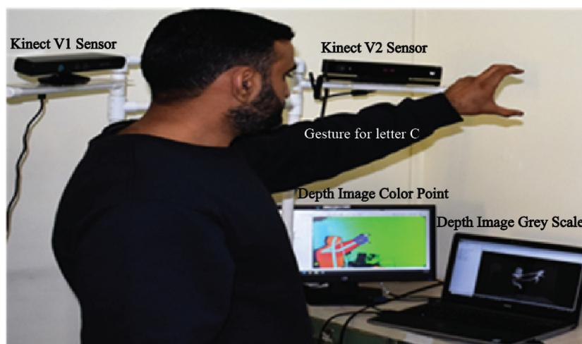
Figure 2. Data acquisition setup for development of case study.
