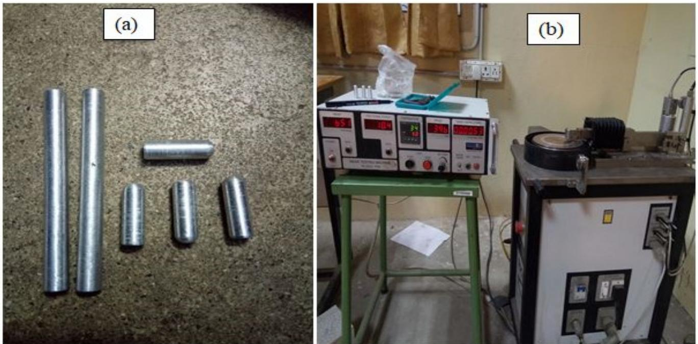
**Figure 12.** Machining product and pin-on-disc setup (a) test specimen, (b) POD test set-up.
