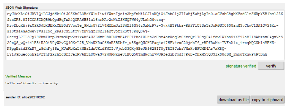
Figure 17. Browser plugin IBS verifying an example. The user verifies a JWS, which supports message recovery and obtains the signed message as well as the signer's public identity.
