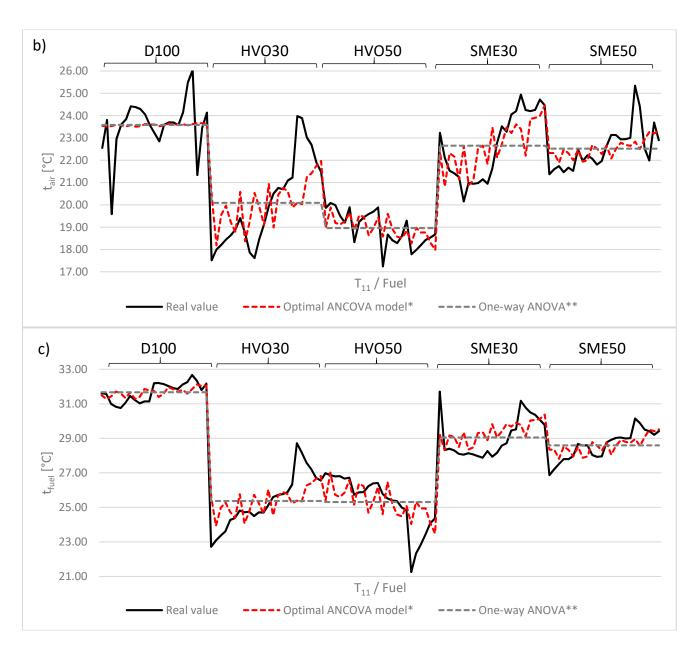
**Figure 6.** Engine exhausted emission real and prognostic values for (a)  $NO_X$ , (b)  $t_{air}$  and (c)  $t_{fuel}$ . Optimal ANCOVA model prognosis was made form Equation (2) and Table 8 parameter estimates. One-way ANOVA prognosis was made form one-way ANOVA with only power or type of fuel predictor.
