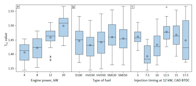
**Figure 4.** Distribution of time domain parameter  $T_{11}$  calculated from TRAV<sub>1</sub> by (**a**) Engine power, (**b**) Type of fuel, and (**c**) Injection timing.
