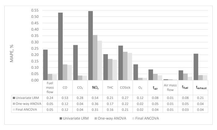
**Figure 5.** Mean absolute percentage error for exhausted emission parameters calculated from univariate linear regression model (LRM), one-way ANOVA and final ANVOVA.
