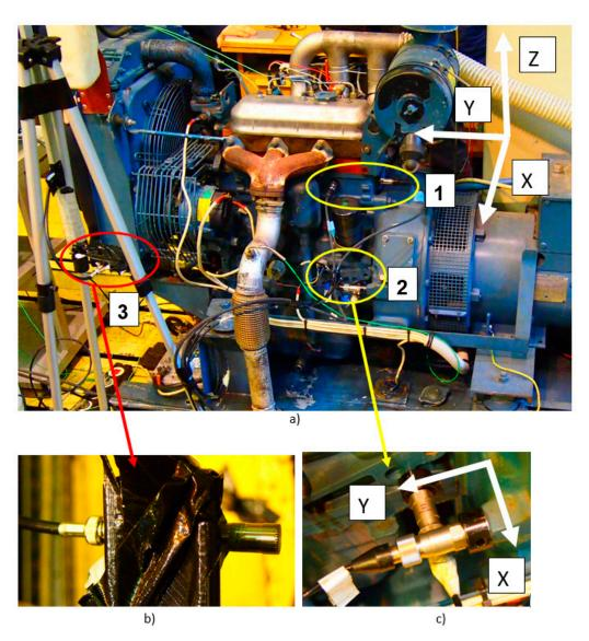
**Figure 3.** Points of measurement of vibrations and sound pressure: (a) general view of the engine being analyzed and points of measurement of vibrations (points 1 and 2) and sound pressure (point 3); (b) a microphone to measure sound pressure (point 3); (c) accelerometers to measure vibrations (point 2) in X and Y directions.
