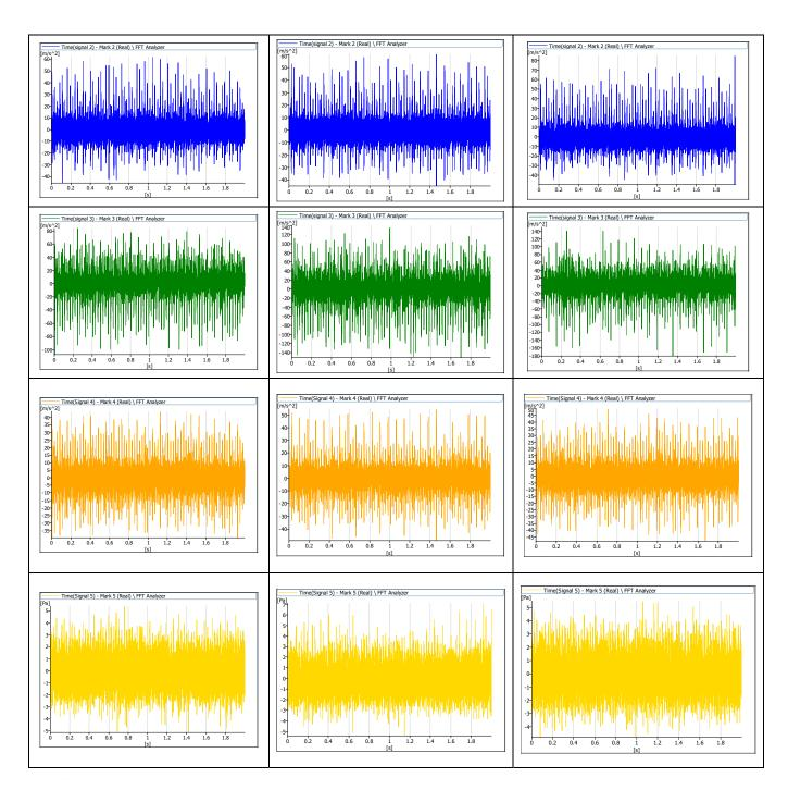
**Figure A1.** Typical results of measurement of vibrations and sound pressure (D100, HVO50 and SME50) under 20 Nm load and injection timing 10 CAD BTDC.
