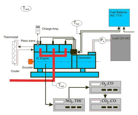
Figure 1. The engine test system.
