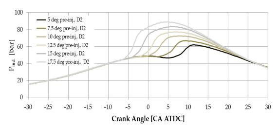
**Figure 2.** The measured injection tube pressure and the in-cylinder pressure (indicated) pressure in the function of the crank angle at 20 kW load and D2 fuel.
