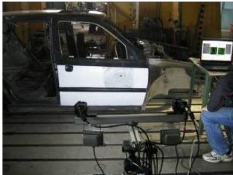
Figure 23. Door surface monitoring with VIC-3D system.
