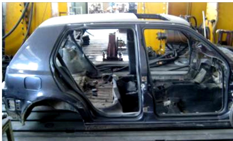
**Figure 13.** The car body used on the stand.
