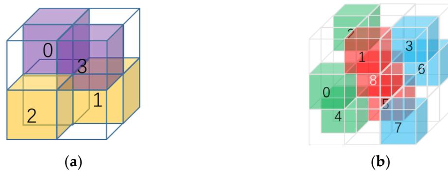
**Figure 1.** Two types of fractal models. (a) Type I: fractal model sized  $2 \times 2 \times 2$ ; (b) Type II: fractal model sized  $3 \times 3 \times 3$ .
