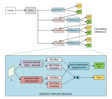
**Figure 1.** Region proposal networks and Cascading Grid Region Convolutional Neural Networks (RCGrid R-CNN) architecture.
