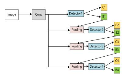
Figure 5. The architecture of the cascading detector modules.
