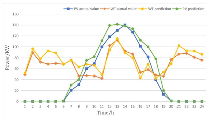
**Figure 10.** The predicted and actual value of WT and PV in Scenario 1.
