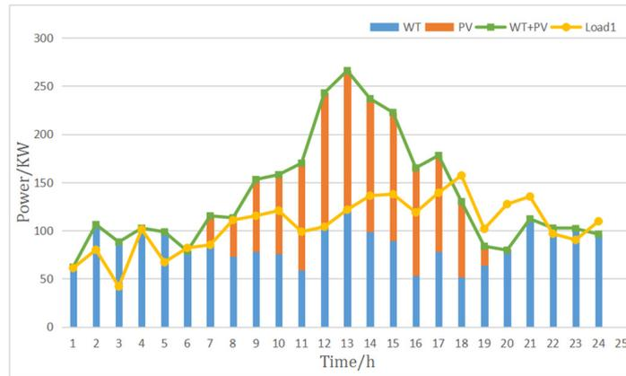
Figure 11. The best output under constraints in Scenario 1.
