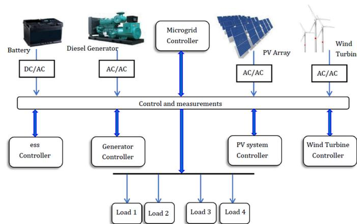
Figure 1. Basic structure diagram of islanded microgrid.
