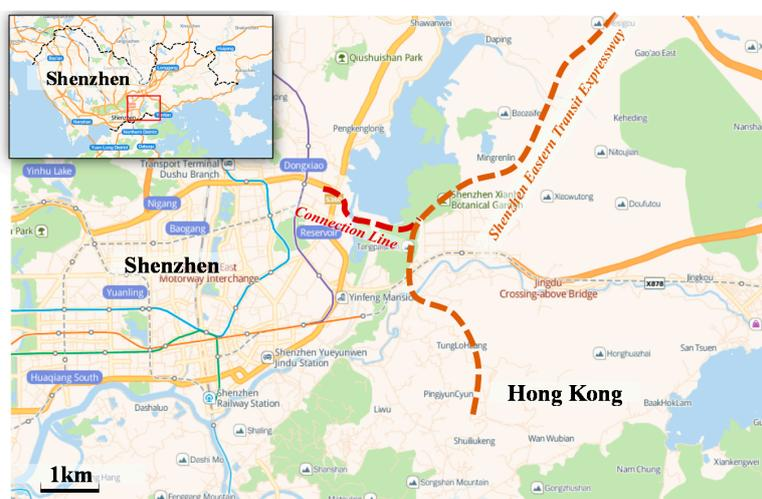
Figure 1. Route plan of the Shenzhen Eastern Transit Expressway Connection Line.
