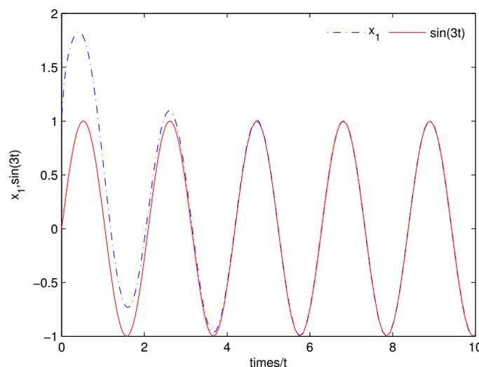
Figure 3. Shows the state  $x_1$  of the system (22) converges to  $c(t) = \sin(3t)$  as  $t \rightarrow \infty$ .
