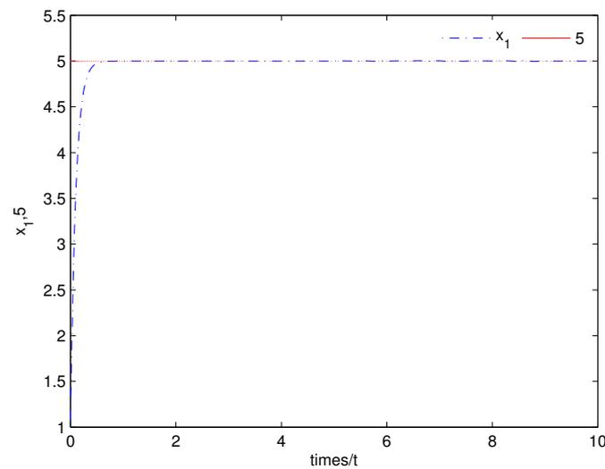
**Figure 1.** Shows that the state  $x_1$  of the system (15) converges to  $c(t) = 5$  as  $t \rightarrow \infty$ .
