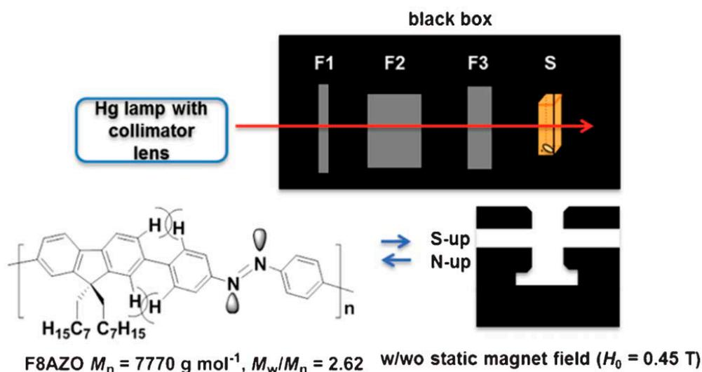
**Figure 19.** Schematic representation of setup for CPL triggered chirality induction and modulation in a solution of F8AZO particles by r-/l-CPL (reprinted with permission from Reference [83]. Copyright 2013 The Royal Society of Chemistry).
